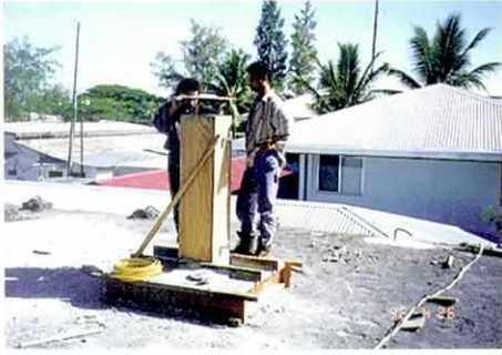
Photo 7. GPS antenna at the roof top of the Palau Bureau of Lands and Surveys.
