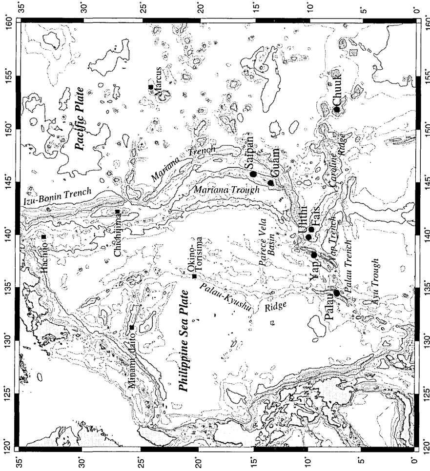
Fig. 6-2. Ocean bottom topography of the Philippine Sea and GPS site locations. Circles denote the Philippine Sea Plate campaign sites and squares continuous observation sites in this area except Okino-Torishima which is the other campaign site.
