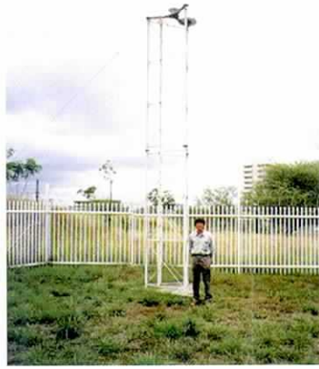
Photo 8. GPS antenna tower at the Port Moresby site established at the PNG National Mapping Bureau.
