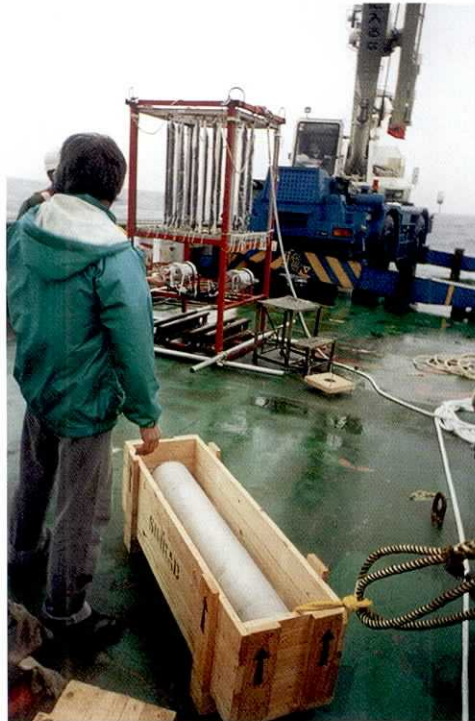
Photo 1. Whole scape of Kongsberg Simrad SWB 600 before experiment. The cylindrical metal in the wooden box is a magnesium anode.
