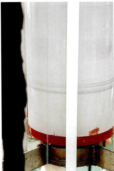
Photo 4. Anode surface after experiment 2. White material on the anode surface is hydrated Magnesium.
