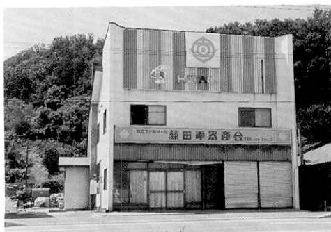
Photo 11. Fujita electric shop, the lower part of shutter plates were slightly damaged. Sea water rose up to the pointed level by Mr. A. Satake.
