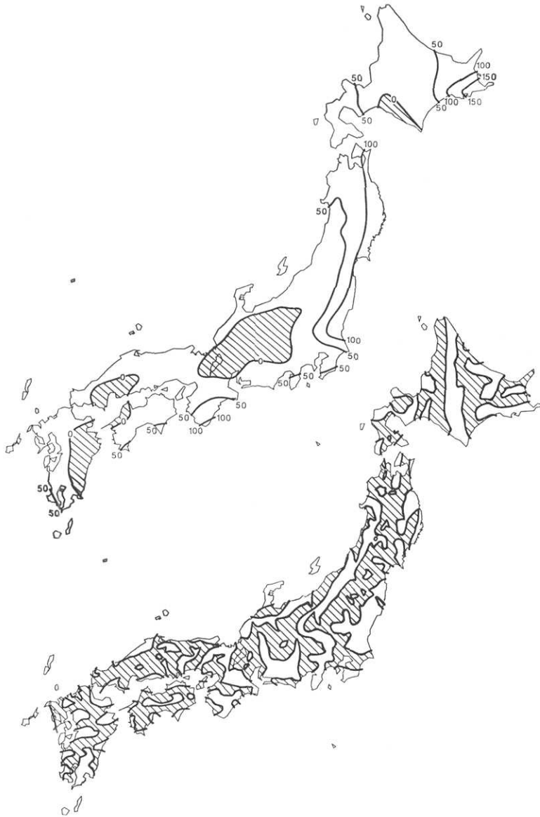
Fig. 7. Bouguer anomaly distribution of long (a) and short (b) wavelength in Japan. Hatched regions show negative Bouguer anomalies (after HAGIWARA, 1967). Contour interval is 50 mgal.
