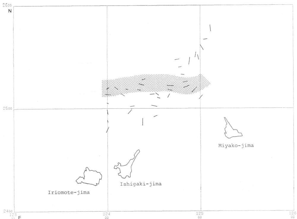
Fig. 11. Linearity and directions of the magnetized body calculated from the geomagnetic three components measured by STCM in the southwestern part of the Okinawa Trough. Hatched area shows the location of the Yaeyama Graben in the trough.
