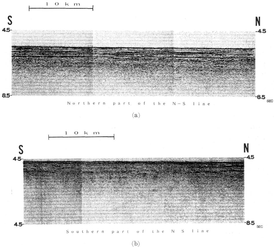
Fig. 3. Image of seismic profiling digitally processed along the N-S seismic survey line A of Fig. 1. Entire line is divided into two sections. a: northern section and b: southern section. The vertical scales are two-way acoustic travel time in seconds.
