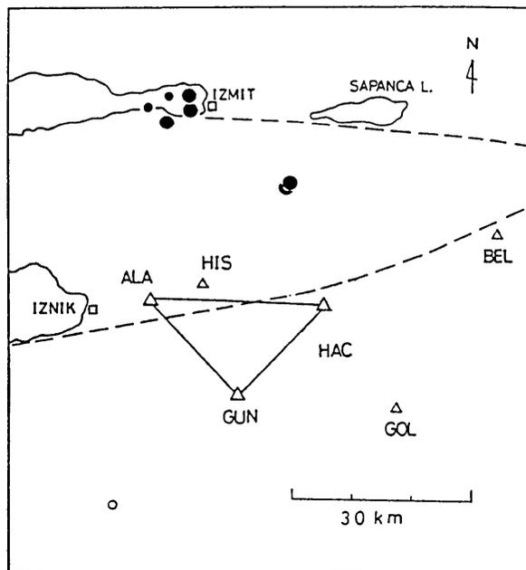
Fig. 3. Map showing seismic stations (open triangles) and epicenters determined by data from the three stations ALA, HAC and GUN. Large and small solid circles indicate earthquakes with magnitudes greater than and smaller than 2, respectively. Open circle denotes explosion. Broken lines denote fault traces: the Iznik-Mekece Fault (lower) and the Iznik-Sapanca Fault (upper).
