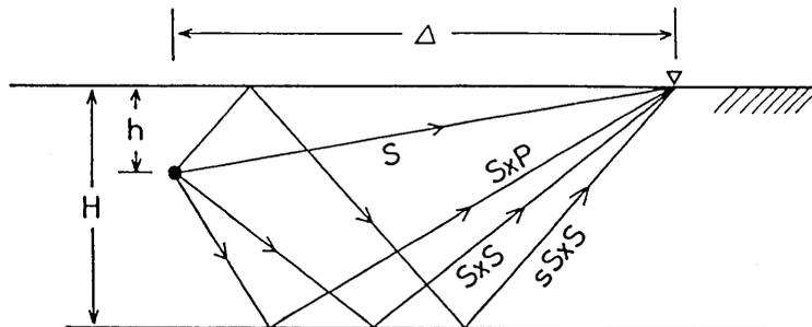
Fig. 16. Ray paths from a source to a station for various reflected waves.
