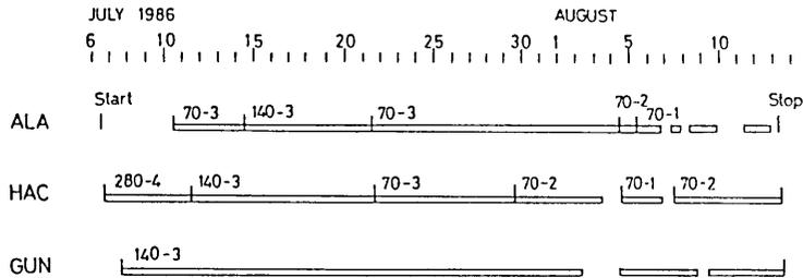
Fig. 4. Sensitivities and threshold levels for tripartite stations. The box shows the operation period. The numerals indicate the sensitivity in  $\mu$  kine/mm (left) and the threshold level in the unit of sensitivity (right).
