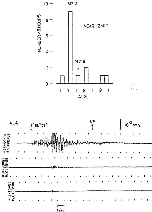
Fig. 7. Number of swarm earthquakes detected at ALA, for every 6 hours, and the waveforms recorded at ALA. The source area is around Izmit City.
