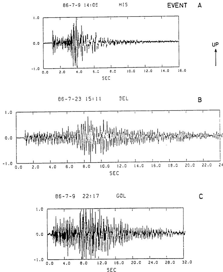
Fig. 10. Waveforms of local earthquakes recorded on the OM-2 cassette recorder. Amplitudes are normalized by the largest one for each event. Event A: The unique local earthquake with a small S-P time less than 5 sec recorded on this recorder. Event B: One of the clustering events near Izmit City. Event C: The earthquake that took place about 55 km east of GOL, judging from P and S times at GOL and GUN as well as the routine hypocentral data of MARNET at Kandilli Observatory.
