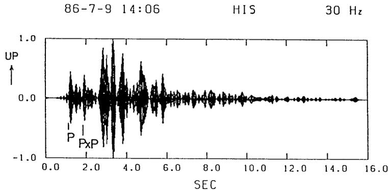
Fig. 15. Filtered seismogram of Event A for a 30 Hz band. Direct *P* and the corresponding *PxP* phases are identified.
