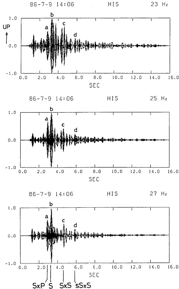
Fig. 14. Filtered seismograms through recursion digital filters without phase-delay for Event A shown in Fig. 10. The frequency bands are designed by  $(0.909f, 1.1f)$ , where  $f$  is the center frequency given in the figure. The frequency giving half of the amplitude is  $1.2f$ , i.e., the decay rate being 48.4 dB/oct. Interpreted reflected arrivals are indicated by their symbols.
