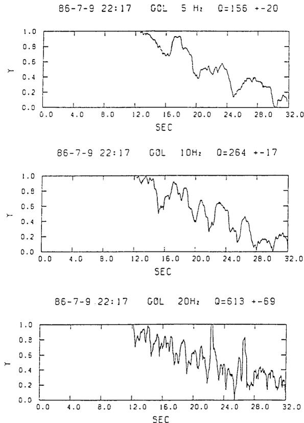
Fig. 11. Example of modified smoothed coda amplitude curves defined by equation (4) as a function of time for different frequency bands. The time axis is common with Fig. 10 (Event C). The amplitudes are normalized by the maximum.
