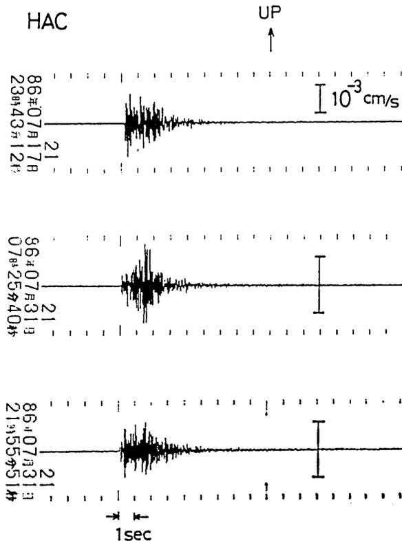
Fig. 6. Waveforms of ultra-microearthquakes recorded at HAC.
