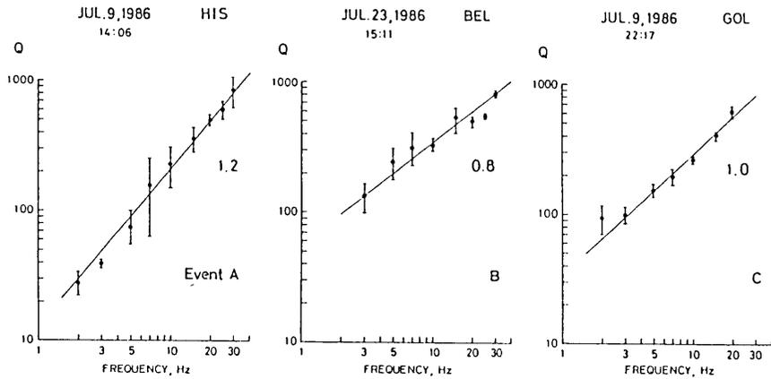
Fig. 12. Coda  $Q$  values as a function of frequency. Their frequency dependence is approximately expressed by  $Q \propto f^r$ , which is shown by straight lines. Numerals indicate the values of  $r$ . The error bars are obtained by taking the standard deviation of  $Q$  values calculated for 11 different time windows (See text).
