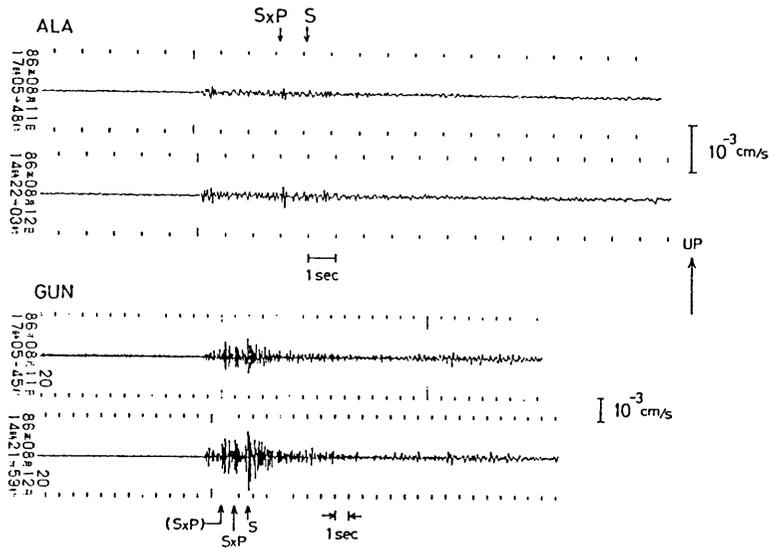
Fig. 8. Examples of waveforms of a series of explosions originating 30 km southwest of GUN. Two epicenters are determined as shown in Fig. 9(a).
