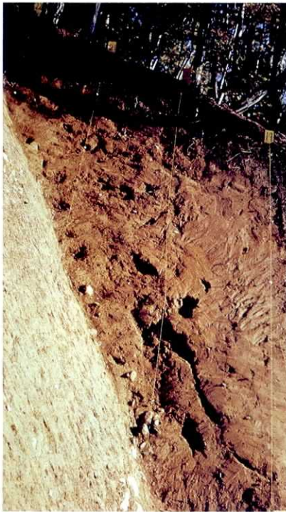
—Fig. 28. Cracks observed in the bed 2a at East wall of trench A.
