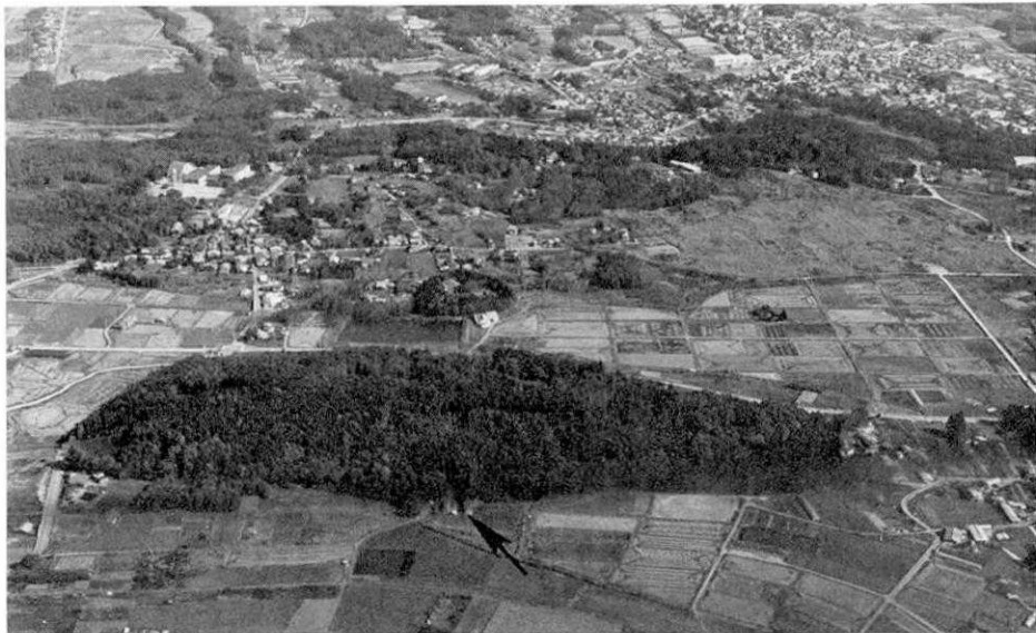
Fig. 6. Oblique airphoto of Nakayama hill, a bulge striking northwestward. Arrow indicates the location of trench A on the Wakamiya Fault, which was geomorphologically estimated to be located on the base of the western slope of the hill. Above: slope of Yatsugatake Volcano.
