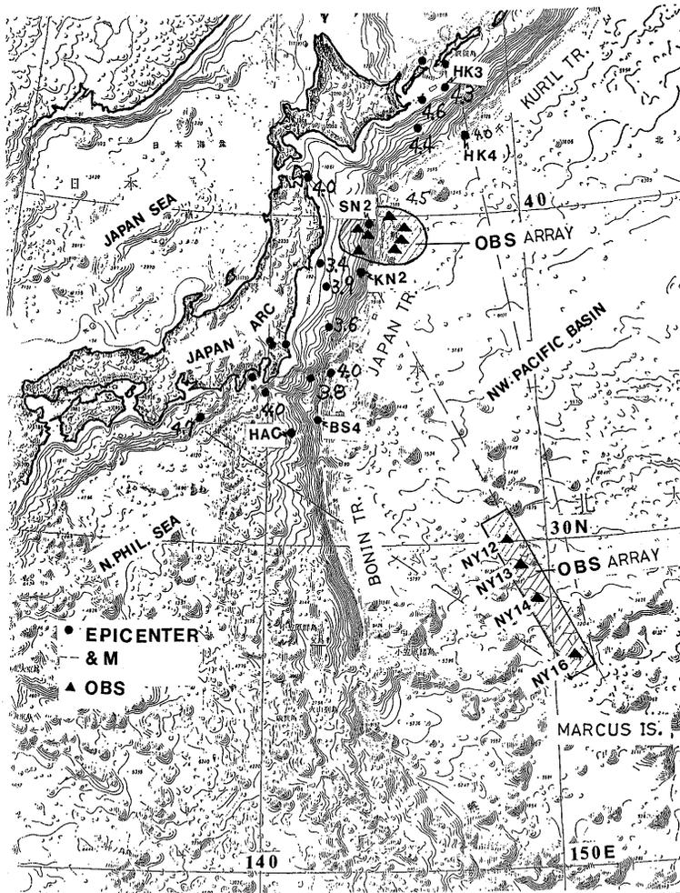
Fig. 1. Locations of OBS (Ocean-Bottom Seismometer) array (solid triangles) and epicenters of natural earthquakes (solid circles). The one array deployed far off Northeast Japan is for increasing the accuracy of the earthquake source data, and the other array deployed southeasterly towards Marcus Island is for covering long range observations. The record sections are made for 6 earthquakes HK3, HK4, SN2, KN2, BS4 and HAC.
