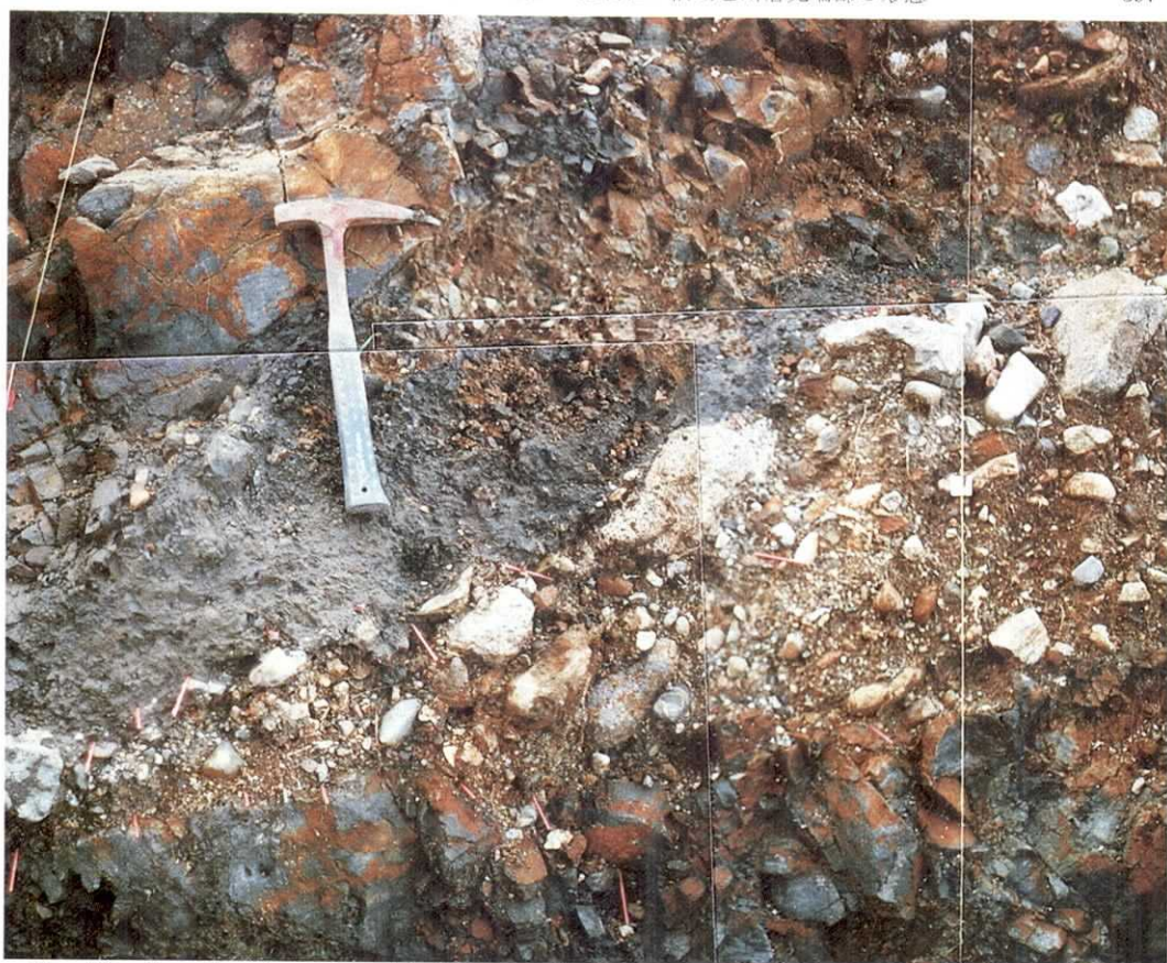
Fig. 35. Gravel wedge intercalated tectonically between mudstones on hanging-wall and footwall of F fault on NS-wall. The upper margin of the wedge is bounded with F fault and contacts with crushed mudstone. The base of the wedge is an unconformity.
