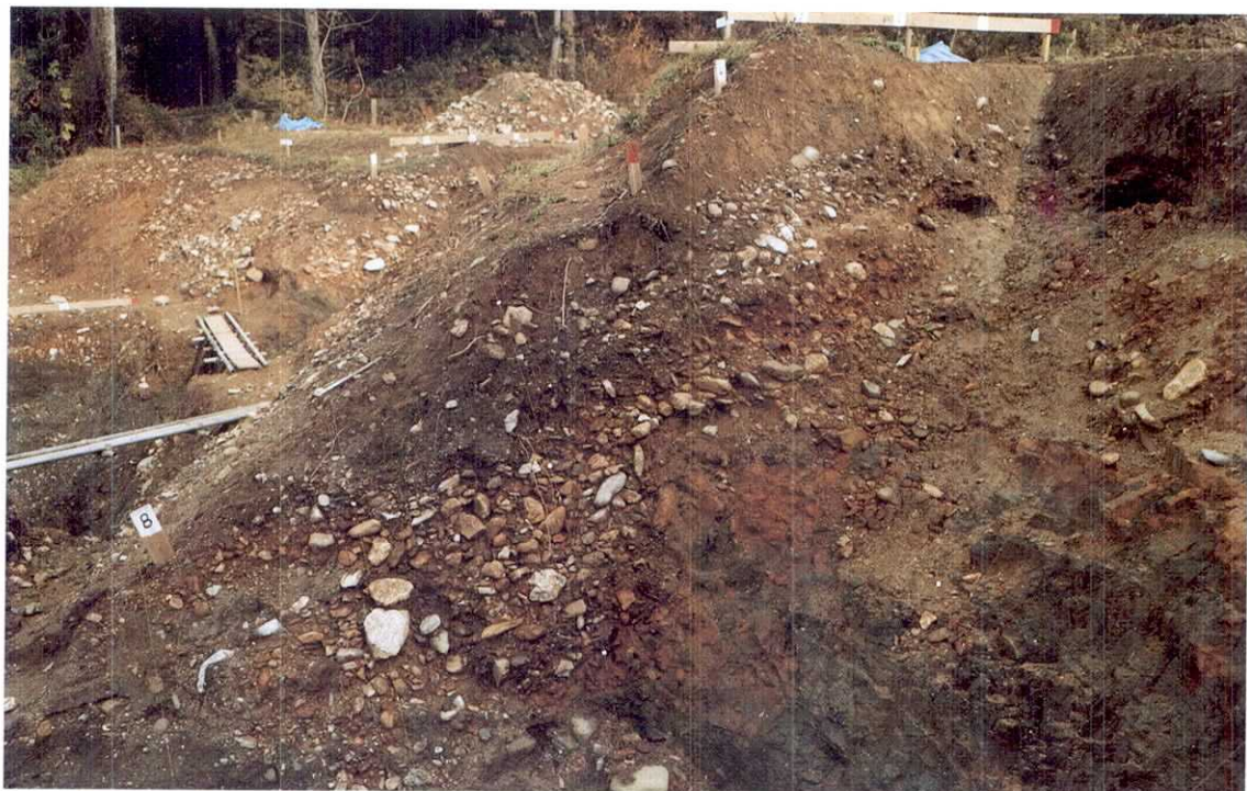
Fig. 33. MN-wall. Gray mudstone with reddish margin is on the hanging wall of F fault (The sketch is in Figure 11A).
