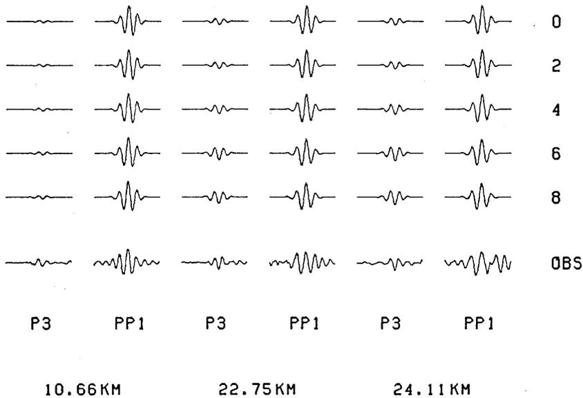
Fig. 4. The progression of ray-theoretical waveforms from the starting model through eight iterations. The observed waveforms are shown at the bottom with letters OBS.
