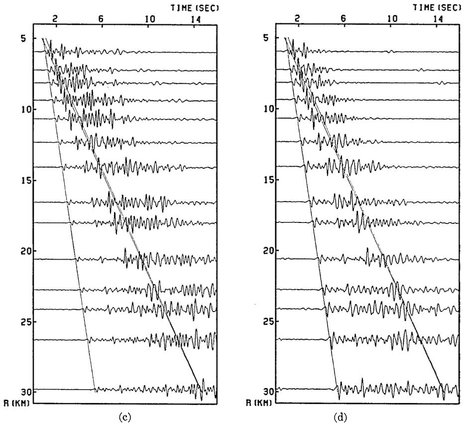
Fig. 3. Synthetic record sections computed with the  $Q_P$  of the surface layer equal to (a)  $\infty$ , (b) 100, (c) 50 and (d) 20.
