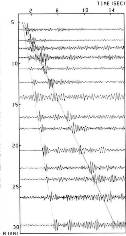
Fig. 2. Observed record section of the first Yumenoshima refraction experiment. Thin solid lines indicate travel times of  $P_3$ ,  $P_0$  and  $PP_1$ .
