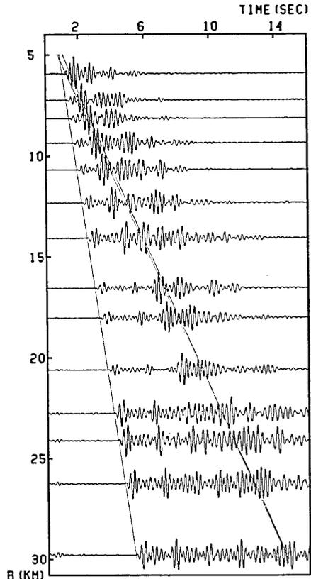
Fig. 5. Synthetic record section computed with the obtained  $Q_P$ -values and the  $Q_S$ -values by YAMAMIZU *et al.* (1983).
