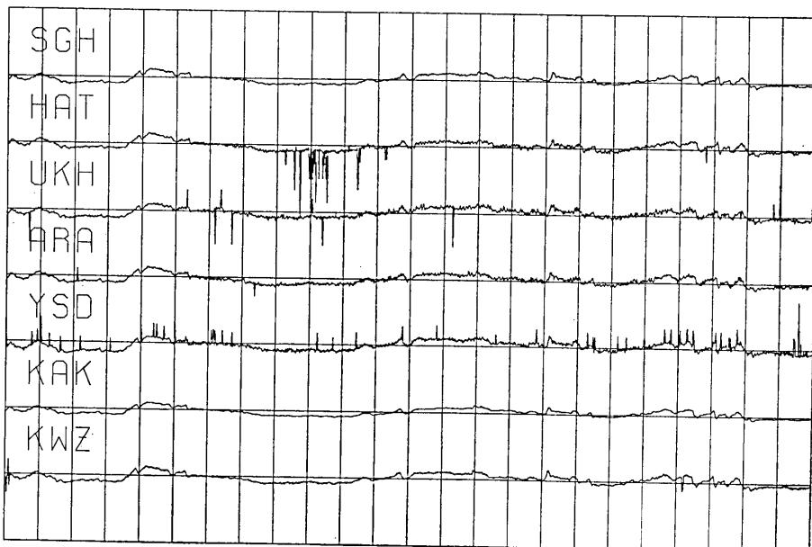
Fig. 2. An example of simultaneous records of total field magnetograms. The vertical spacing corresponds to 100 nT.
