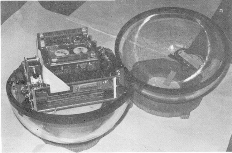
Fig. 1. External view of DOBSH (Digital Ocean Bottom Seismometer and Hydrophone). Recorder, batteries and seismometers are mounted in a 40 cm diameter glass sphere. Debugging unit is not shown.
