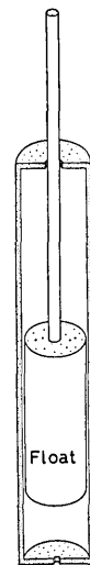
Fig. 6. Schematic cross section of a tide gage tube used in the present study.
