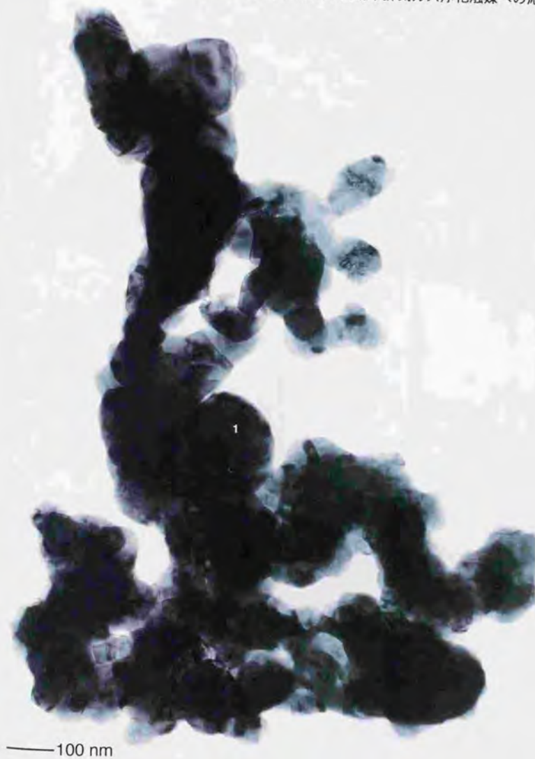
Fig. 5-32. TEM images of Pd/perovskite catalyst aged at 1050 °C for 60 h in engine exhaust gases.
