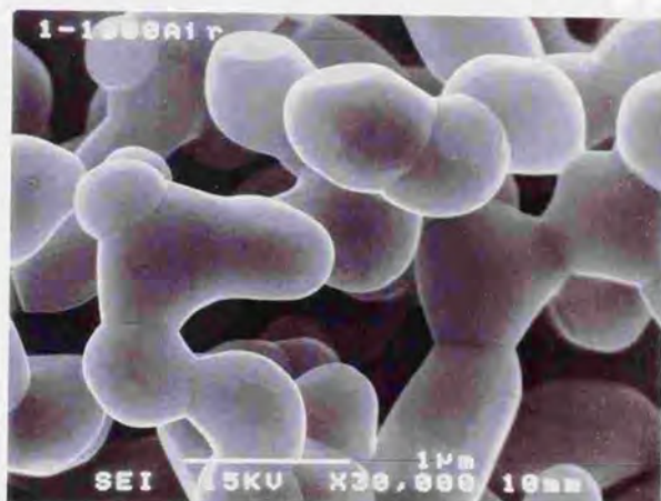
Fig. 6-16. FE-SEM images of \text{LaCoO}_3 aged at 1000 °C for 4 h in air.
