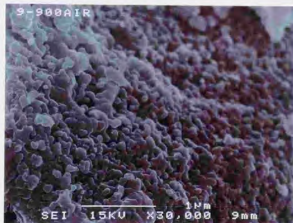
Fig. 6-22. FE-SEM images of \text{LaFe}_{0.54}\text{Co}_{0.36}\text{Pd}_{0.10}\text{O}_3 aged at 900 °C for 4 h in air.
