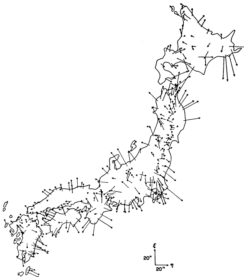
Fig. 8. Astrogeodetic deflections of the vertical with respect to the best suited ellipsoid.
