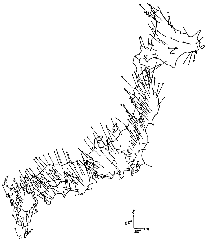
Fig. 6. Astrogeodetic deflections of the vertical in Japan with respect to the Bessel ellipsoid (after the Geographical Survey Institute). Most vectors point to the north-west due to the unsuitability of a reference ellipsoid.
