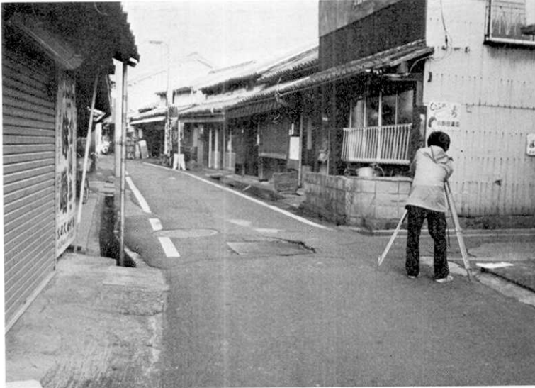
Fig. 6. View of leveling survey of inundation height at Kitamachi, Yuasa.
