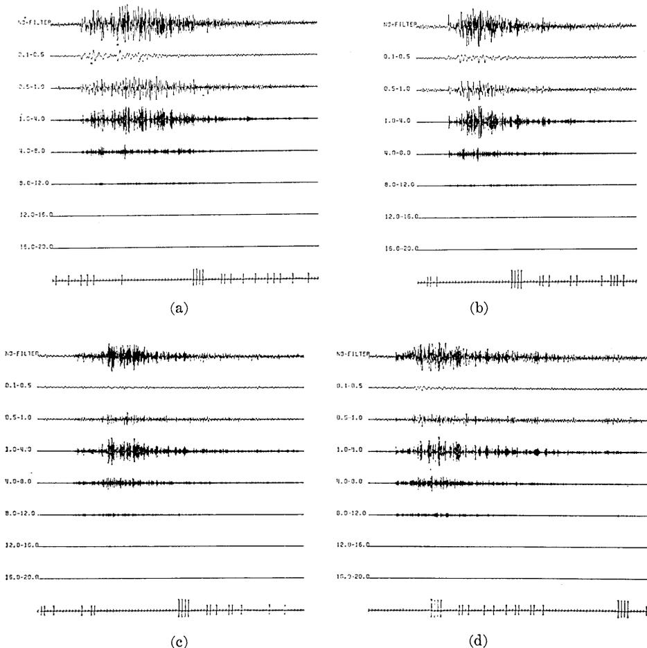
Fig. 9. Chebychev digital band-pass filtering for earthquakes observed at KHQ1. (a) and (b) are low frequency rich. (c) and (d) are less low frequency (0.1-0.5 Hz band). Numbers show frequency in Hz. Comparing 0.1-0.5 and 8-12 Hz, (c) and (d) are high frequency rich, though magnitudes of (a) and (b) are slightly higher than (c) and (d). Bottom trace in each figure shows time code. A tick is one second.
