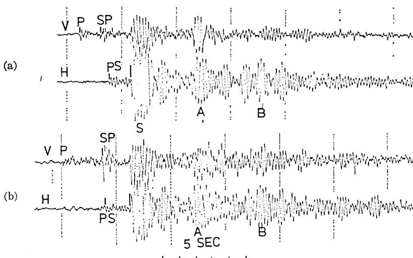
Fig. 11. Expansion records for two earthquakes (a) and (b) which correspond to records (c) and (b) shown in Fig. 10, respectively. When two seismograms (a) and (b) are superposed at first breaks of S-wave, peaks and troughs of phases A and B in (a) are well matched those in (b) each other. Note that initial motions of S-waves on horizontal components are different between two seismograms.
