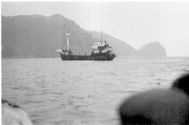
Fig. 4. The No. 16 Seitoku-Maru (200 ton) which was used for laying the submarine cable system.
