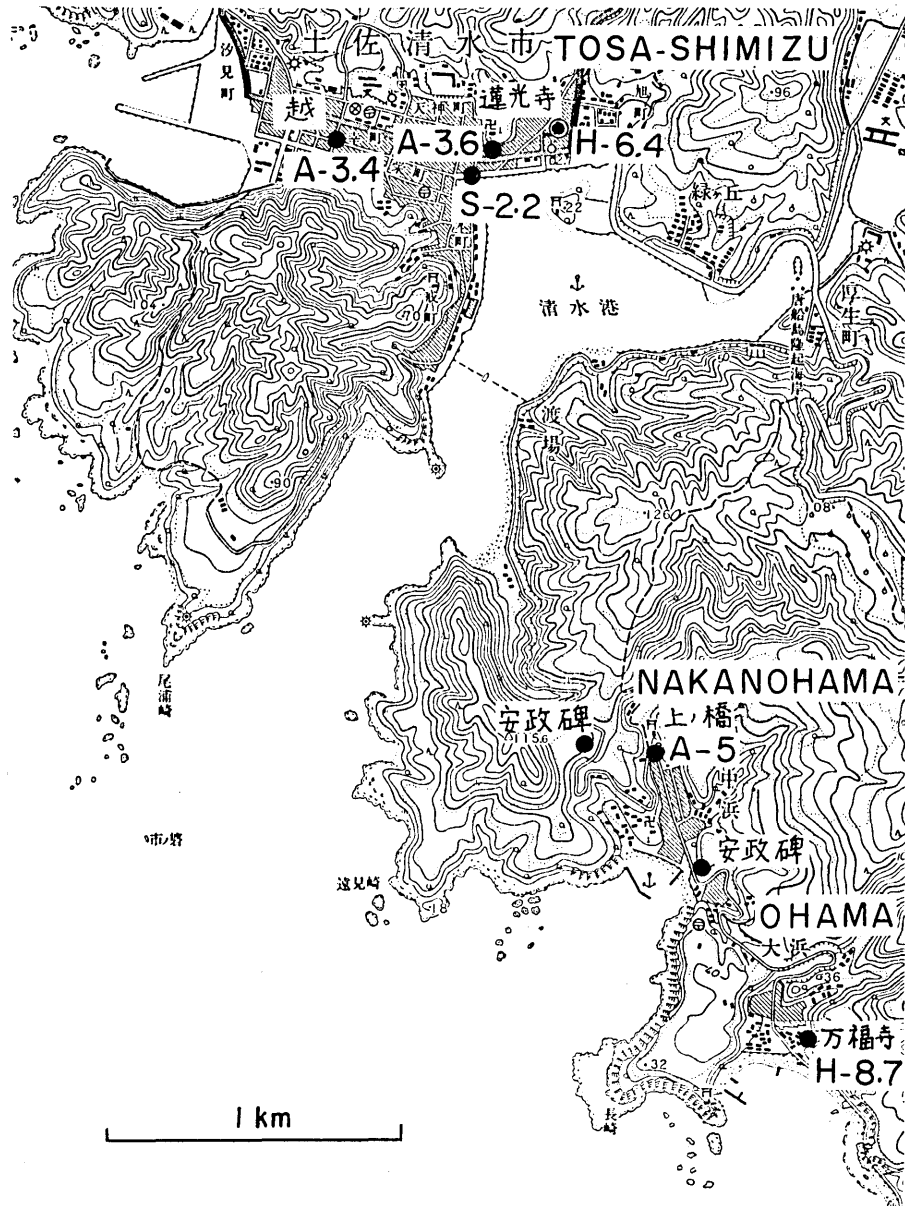
Fig. 7. Inundation heights of the 1707 Hiei (H), 1854 Ansei (A) and 1946 Showa (S) at Tosa-Shimizu (unit: m).
