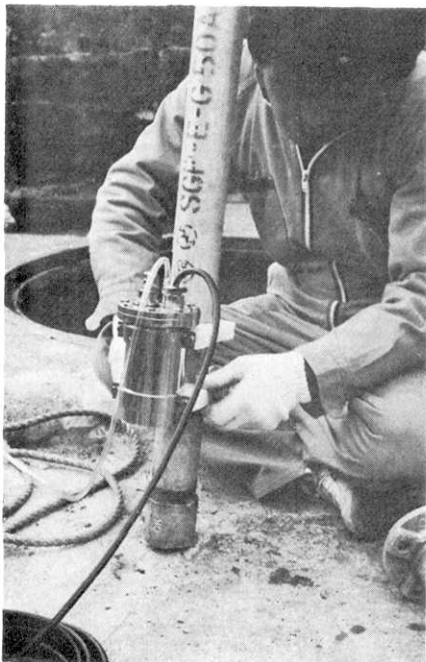
Photo 2. Pressure transducer set on the steel pipe.
