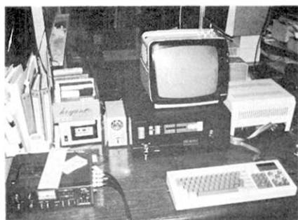
Fig. 3. A snap-shot of the time code reader system.
