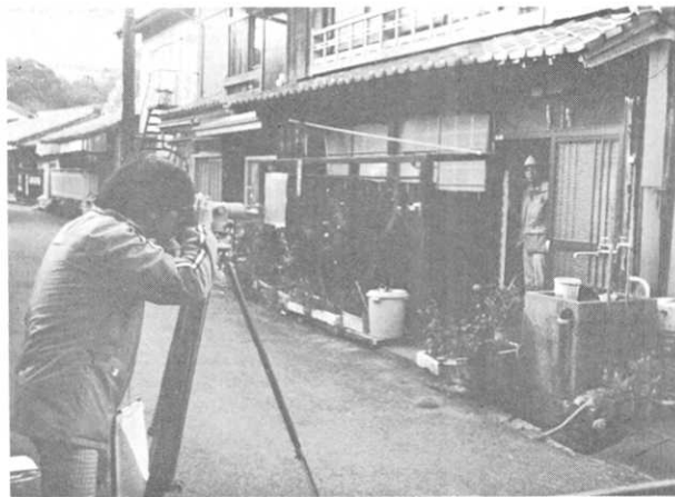
Fig. 3. View of leveling survey of inundation height at Kitaura, Owase.
