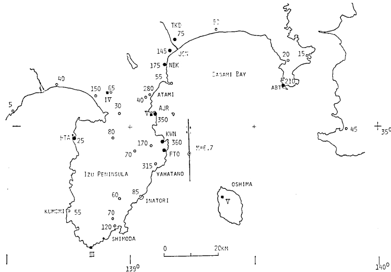
Fig. 1. Map showing the location of strong-motion stations and the observed maximum accelerations for the largest shock (Izu-Hanto-Toho-Oki earthquake) of June 29, 1980. Roman numerals indicate seismic intensities at the JMA stations.
