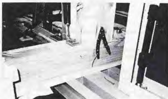
Photo 7. 3. The failure of post-column joint caused by pull-out of the nail in SGBV.
