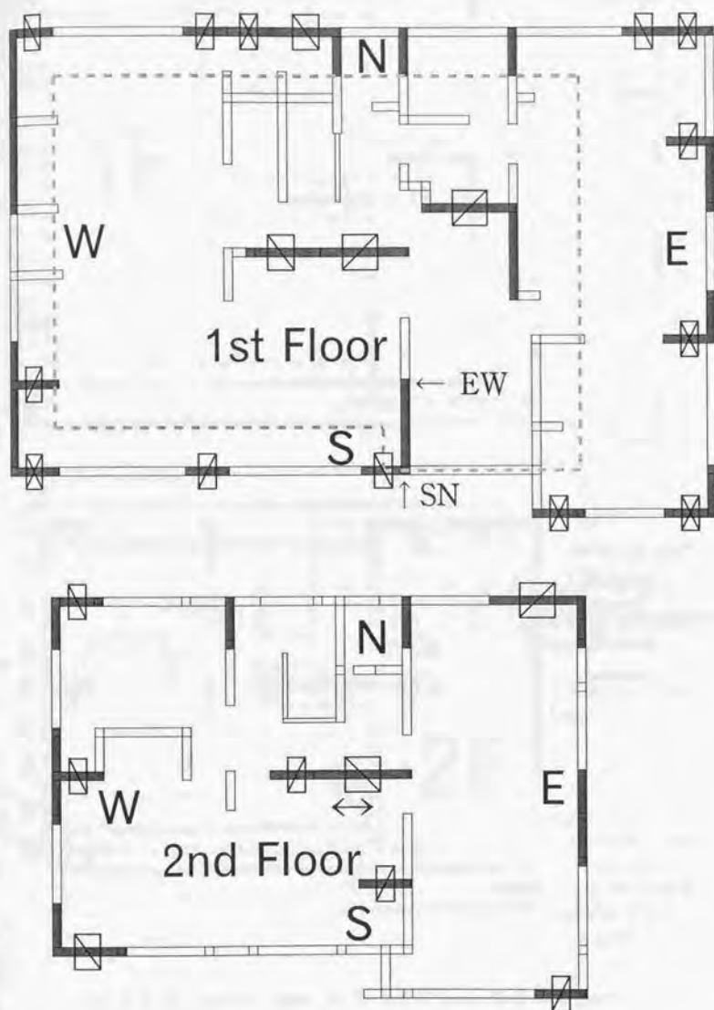
Fig. 8. 2. 2. Schematic plans of the tested house with shear walls layouts of spec. no. 1.
