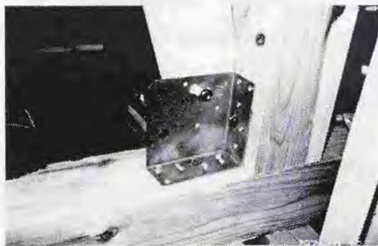
Photo 7. 2. The pull-out of wood screws in SGB.
