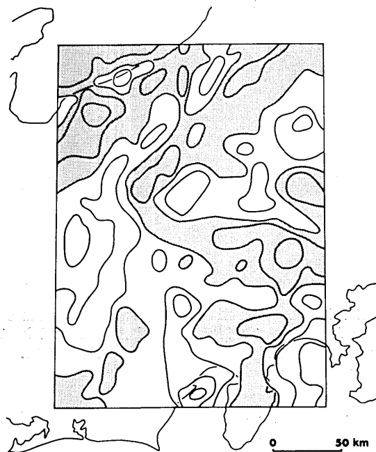
Fig. 4. Pseudototal-intensity anomaly map with a contour interval of 100 nT calculated at the 3 km elevation of the aeromagnetic survey. Stippled area represents a positive anomaly.
