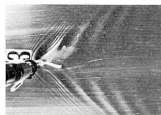
Fig. 12 Effect of fin. Fin width is 6 cm. No oscillation at 20 cm/sec.
