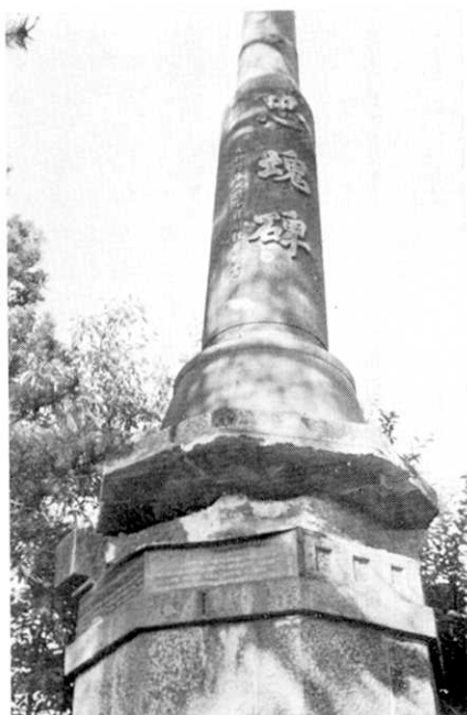
Fig. 14. A monument which broke at the base and rotated by 60 degrees, but did not fall down.
