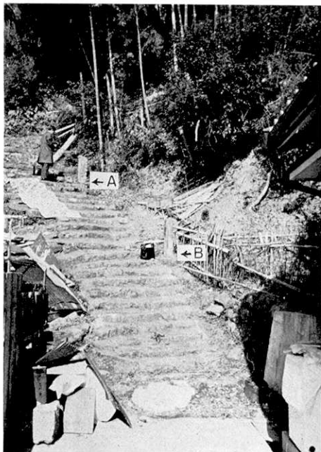
Fig. 19. Inundated sea-levels at Asakawa. A: the 1854 Ansei tsunami. B: the Nankaido tsunami of Dec. 21, 1946. Difference of the sea-levels is 2.3 m.
