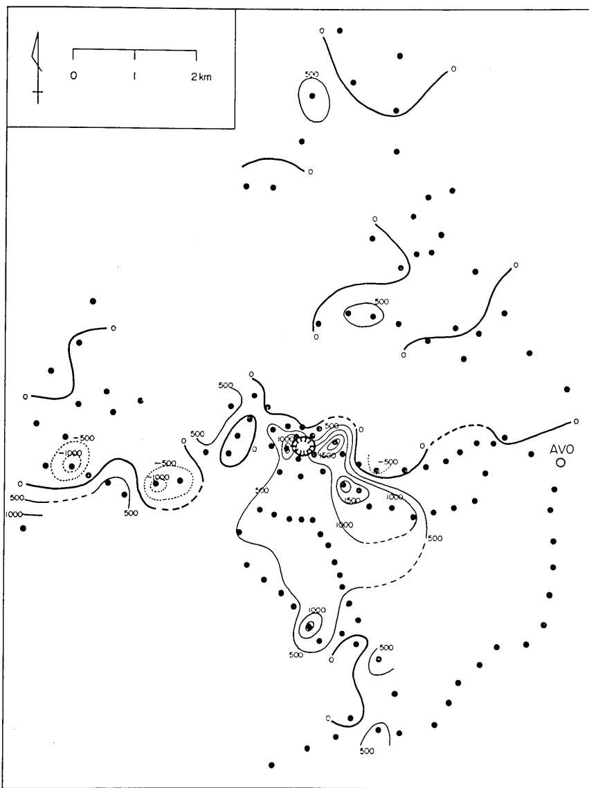
Fig. 3. Magnetic anomalies in the Asama Volcano area. Values are given in gammas.
