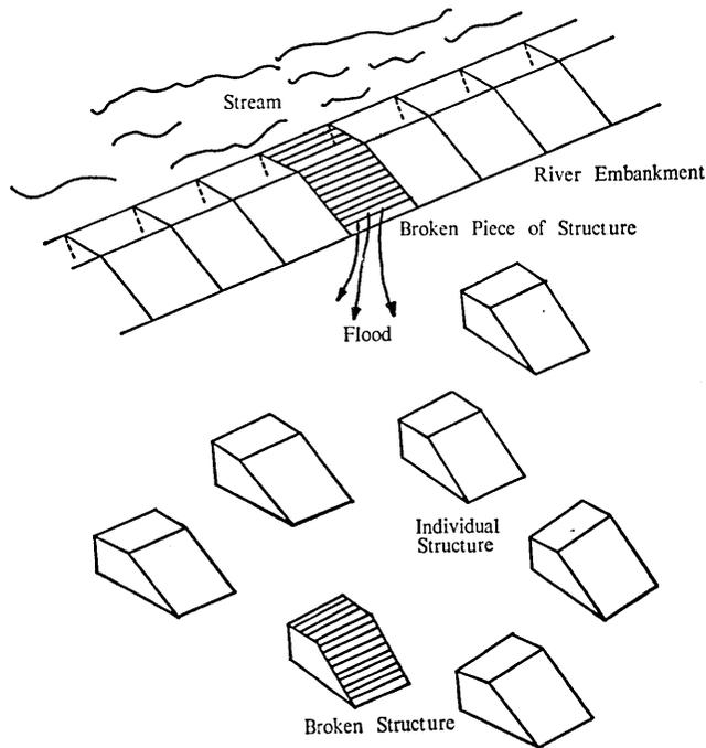
Fig. 1. A failure model of river-embankment.
