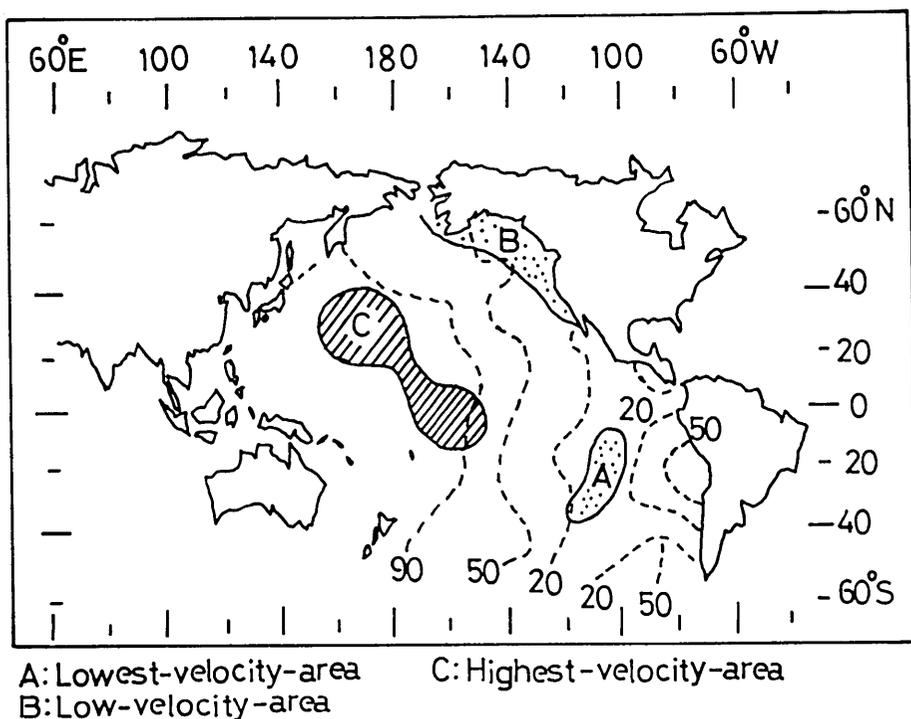
Fig. 4. Map of the group velocity and the ocean-floor age in the Pacific. In the region A the velocity is the lowest and it is the highest in the region C. The velocity in the region B is comparatively low. Dashed curves indicate isochrons 20, 50, and 90 m.y. of the ocean-floor age.
