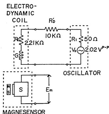
Fig. 4. Schematic circuit diagram for the measurement of  $SG/K$ . The values of the elements shown are those on the experiment.  $R'_b$  is selected so as to give the maximum flat response.
