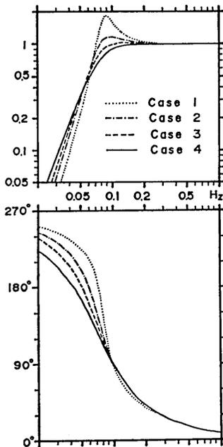
Fig. 6. The change of the characteristics of the seismometer when the corner angular frequency of the amplifier is changed by the change of capacitance. This figure clearly shows that (11) is the necessary condition.
