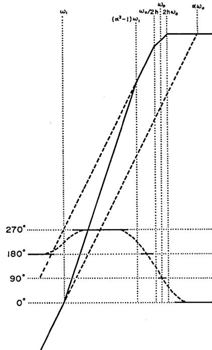
Fig. 3. Outline of the frequency characteristics of PELS with the present device. The upper one and the lower one represent schematic amplitude and phase characteristics respectively.
