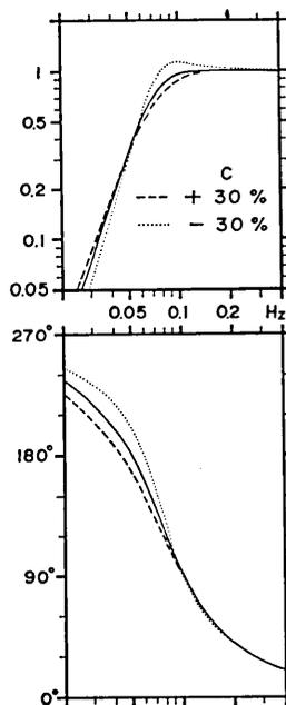
Fig. 9. The change of the characteristics when capacitance in the circuit changes by  $\pm 30\%$ .
