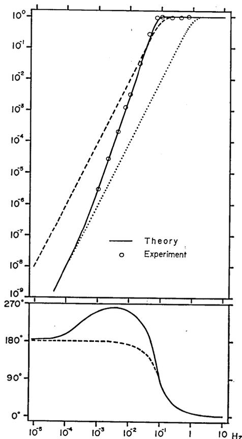
Fig. 5. Rigorous frequency characteristics of PELS with the present device. The upper one and the lower one represent amplitude and phase characteristics respectively. Solid lines represent the theoretical ones and the open circles represent the experimental data. Both are in agreement with each other. Characteristics of 1 Hz's pendulum with  $h = 1/\sqrt{2}$  (dotted line) and 0.1 Hz's pendulum with  $h = 1/\sqrt{2}$  (dashed line) are simultaneously shown.
