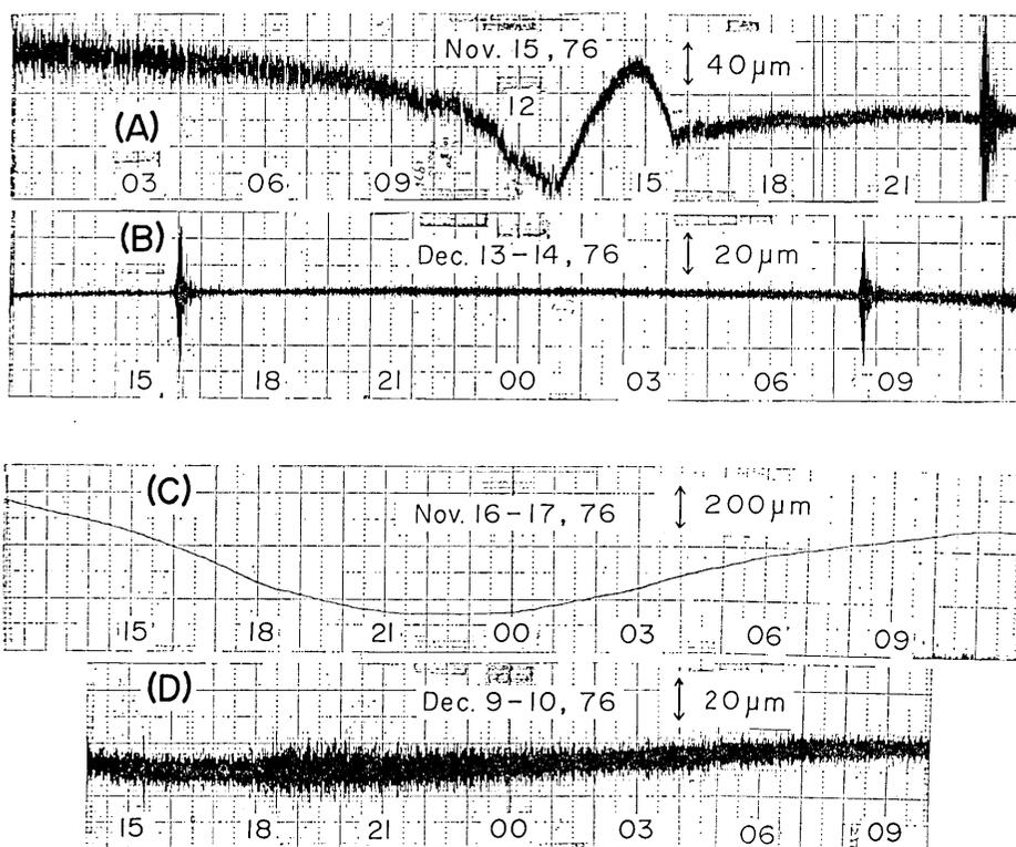
Fig. 10. Examples of the traces. Traces (A) and (B) are horizontal displacements observed with 0.1 Hz's PELS without and with the device respectively. Traces (C) and (D) are vertical displacements observed with 0.1 Hz's PELS without and with the device respectively. Data and time are Japan standard time.
