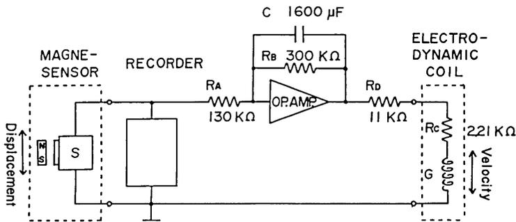
Fig. 1. Schematic diagram of the circuit of the present device. The entered values of the elements are taken from Table 1.
