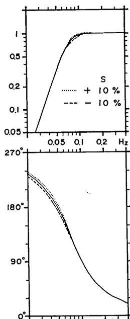
Fig. 8. The change of the characteristics when the  $S$  value changes by  $\pm 10\%$ .
