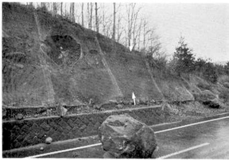
Fig. 70. Outcrop of fault ④ and a fallen block. The surface slope is a part of the fault scarp (Yamanami Highway, 12.5 km, looking east).
