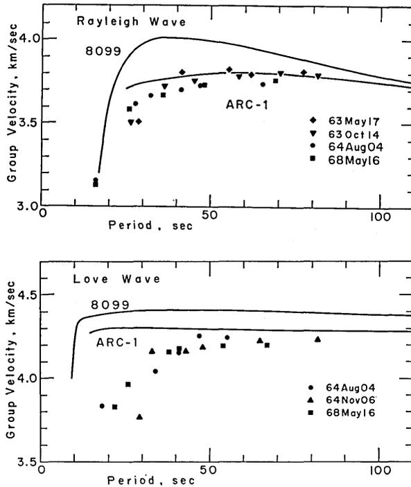
Fig. 2. Group velocities of Rayleigh and Love waves for mixed propagation paths. The dispersion curve of 8099 model fits the normal oceanic data well. The shear-velocity distribution for the two models is given in Fig. 5.
