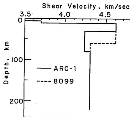
Fig. 5. Shear-velocity model, ARC-1. The oceanic model 8099 which is a starting model in constructing the ARC-1 model is shown for comparison.
