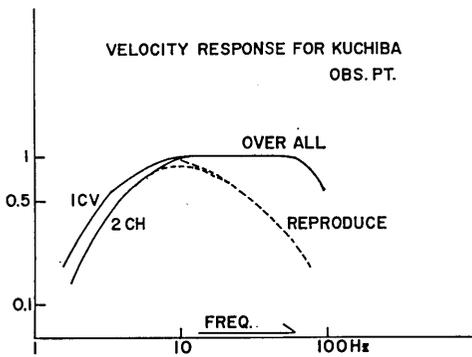
Fig. 7. Frequency response of the instrument installed at KCB. High cut filters are used for reproducing the magnetic tapes.
