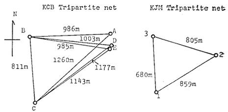
Fig. 6. Relative location of the seismometers of the tripartite nets.
