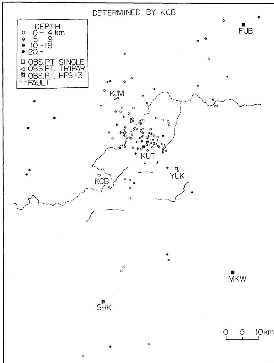
Fig. 17. Distribution of epicenters determined by the KCB tripartite net. Border of prefectures (broken lines) and geological faults (dotted or solid lines) are also shown.
