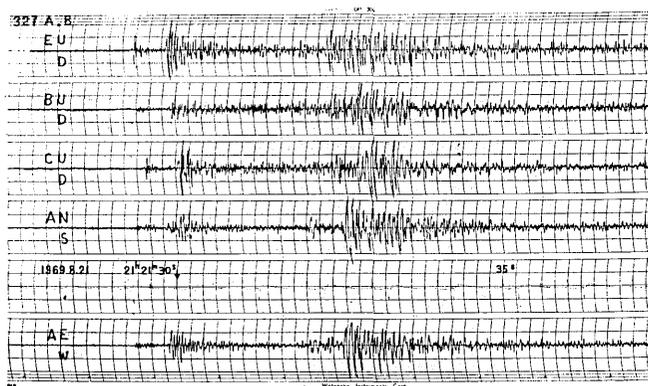
Fig. 23. Seismograms of a couple of earthquakes recorded successively within 0.5 sec at KCB. Locations of the two events are indicated by '—' in Fig. 21.
