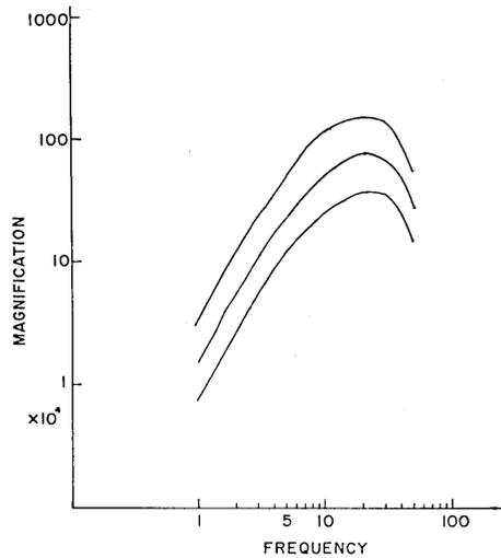
Fig. 8. Magnification curves of the instrument installed at KJM. Magnification is varied according to the ground noise level.
