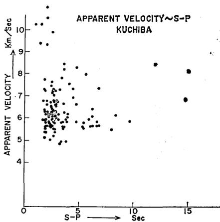
Fig. 15. Apparent velocities versus S-P time intervals at KCB.
