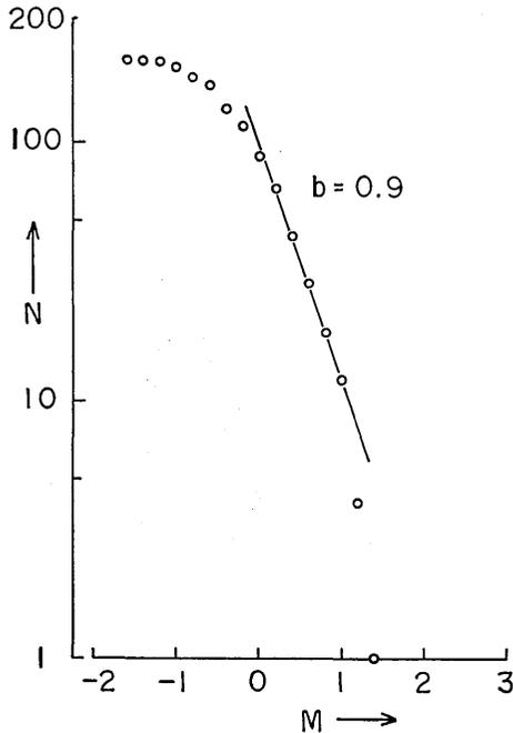
Fig. 14. Cumulative frequency distribution of earthquakes observed at KCB at 0.2 magnitude intervals.
