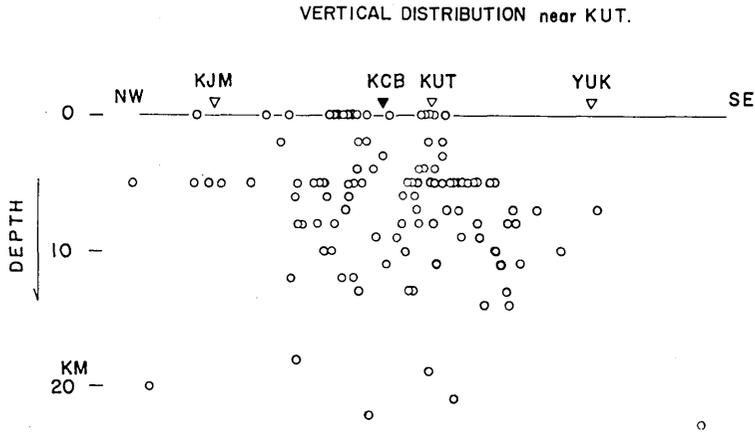
Fig. 18. Projection of the hypocenters on a northwest-southeast striking vertical plane. Earthquakes located in a rectangle whose major axis is in a northwest-southeast direction crossing KUT and minor axis is 15 km in length are plotted in the section.
