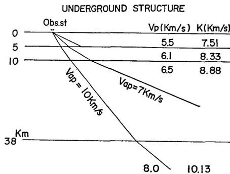
Fig. 16. Underground structure used for location of hypocenters. Referred to Hashizume et al. (1966).
