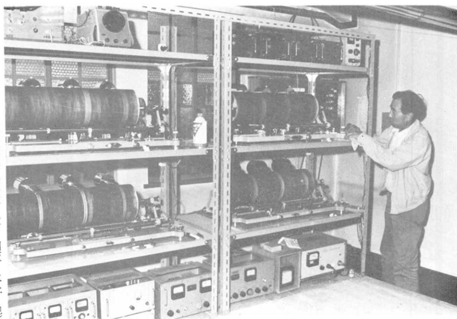
Fig. 31. Smoked paper recorders for continuous seismic observations.
