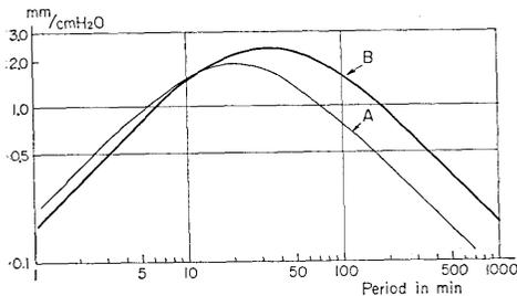
Fig. 3. Spectral response curves of the portable long-wave recorder. A: before improvement, B: after improvement.
