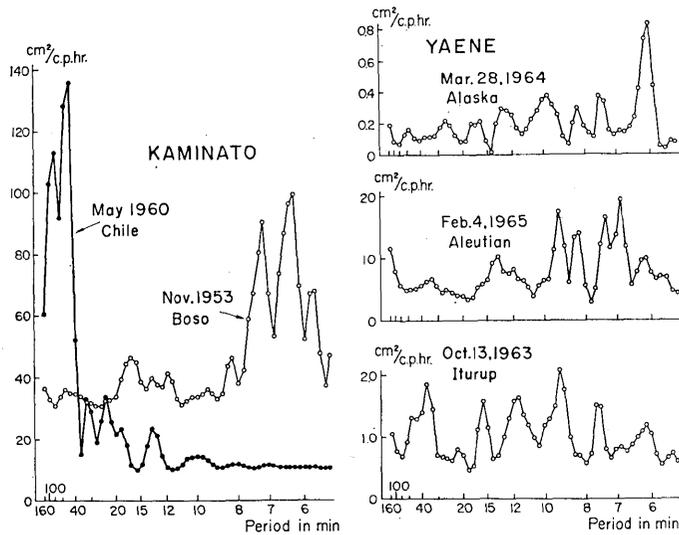
Fig. 10. Power spectra of the different tsunamis observed at Hachijo Island.
