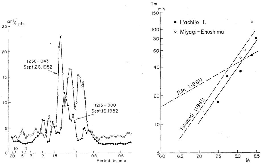
Fig. 11. Power spectra of the tsunamis caused by the eruption of submarine volcano (Myojinsho).
