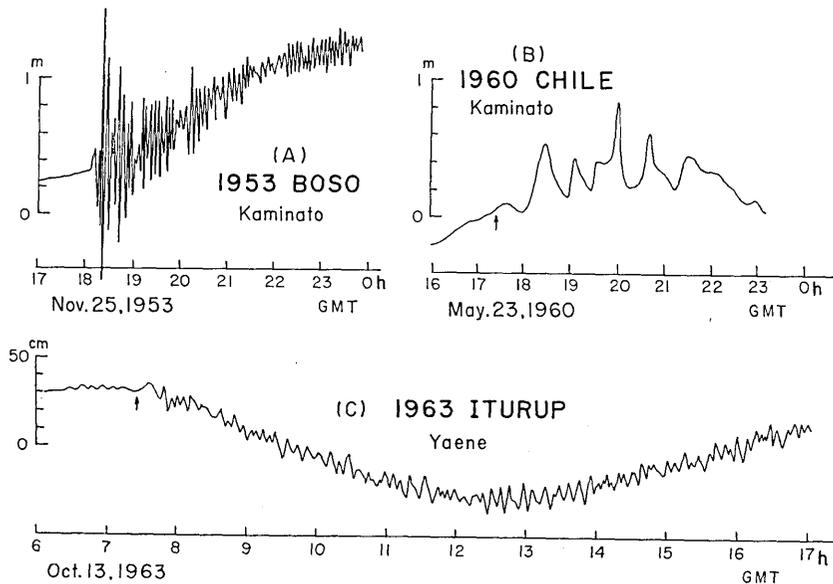
Fig. 8. Records of the different tsunamis observed by tide gauge. A, B: records at Kaminato, C: record at Yaene.
