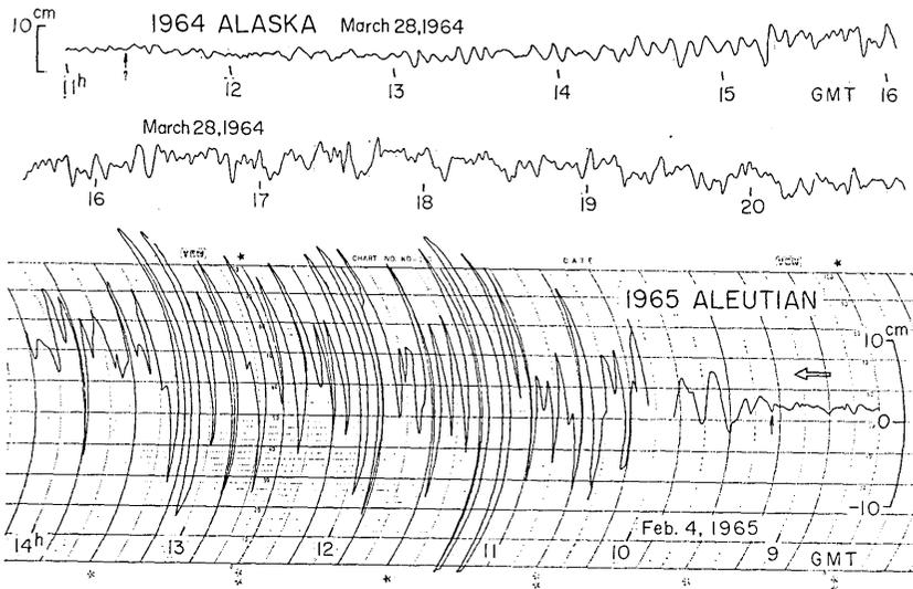
Fig. 9. Records of the 1964 Alaska and the 1965 Aleutian tsunamis observed by the portable long-wave recorder at Yaene.
