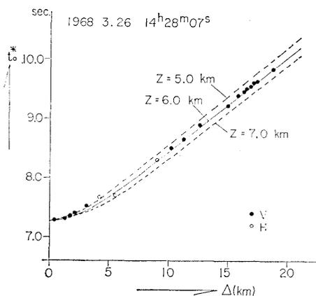
Fig. 15. The travel time curve for the arrival times corrected by the local anomaly of each station and those calculated on the basis of the model structure.
