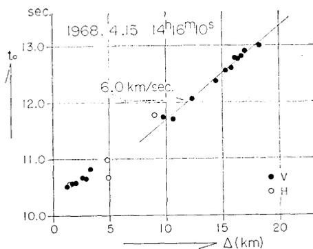
Fig. 12. The travel time curve of the earthquake at 14h 16m 10s on April 15, 1968.
