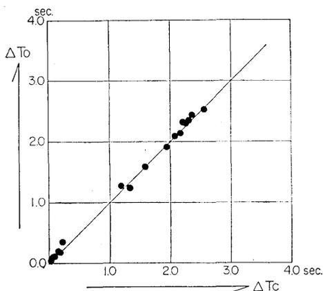
Fig. 16. Comparison of the observed travel time of the earthquake at 14h 16m on April 15, 1968 with that calculated on the basis of the model structure. (hypocentral depth: 5.5km)
