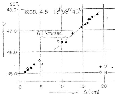
Fig. 11. The travel time curve of the earthquake at 13h 58m 45s on April 5, 1968.
