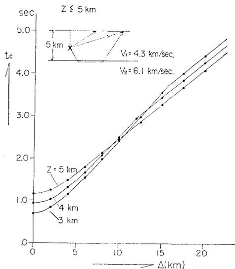
Fig. 13-a. The travel time curves calculated on the basis of the above model structure.
