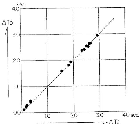
Fig. 19. Comparison of the observed travel time of the earthquake at 16h 46m on March 26, 1968 with that calculated on the basis of the model structure. (hypocentral depth: 6.0km)
