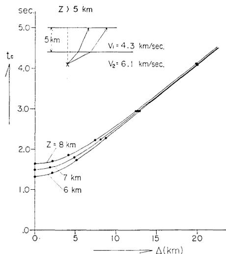
Fig. 13-b. The travel time curves calculated on the basis of the above model structure.
