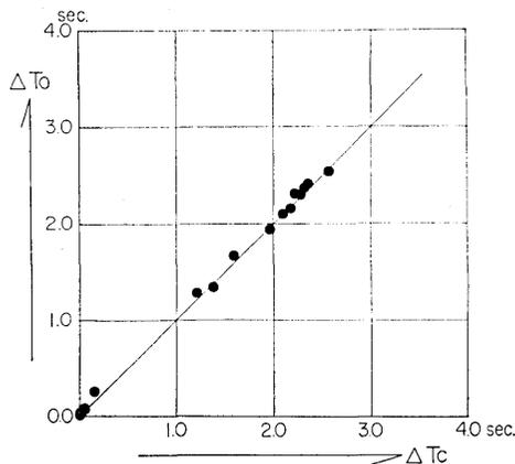
Fig. 17. Comparison of the observed travel time of the earthquake at 14h 28m on March 26, 1968 with that calculated on the basis of the model structure. (hypocentral depth: 6.0km)
