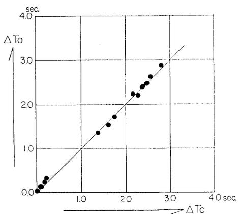
Fig. 18. Comparison of the observed travel time of the earthquake at 15h 51m on March 25, 1968 with that calculated on the basis of the model structure. (hypocentral depth: 5.5km)
