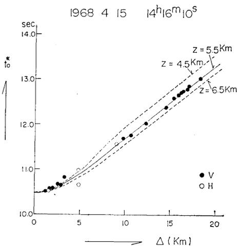
Fig. 14. The travel time curve for the arrival times corrected by the local anomaly of each station and those calculated on the basis of the model structure.
