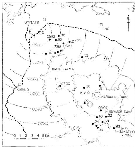
Fig. 3. The coseismal lines of the earthquake at 16h 46m 05s on March 25, 1968.
