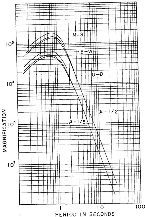
Fig. 1. Magnification curves of HES seismographs.
