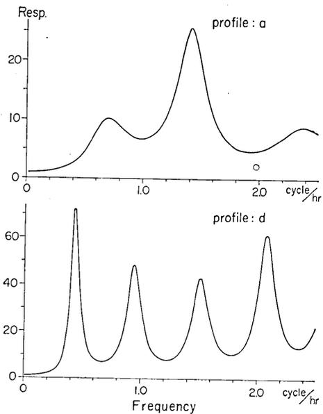
Fig. 3. Response of the continental shelf water in case of the normal incidence of waves.
