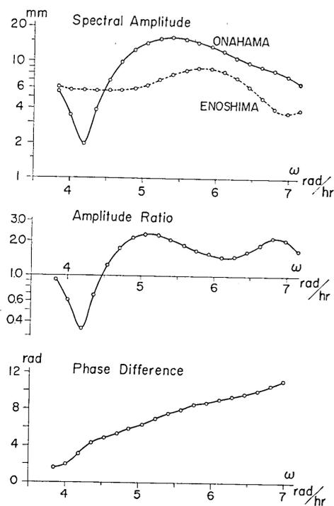
Fig. 9. Results of the Fourier analyses of the records observed at Enoshima and Onahama in case of the Iturup tsunami of 1958.
