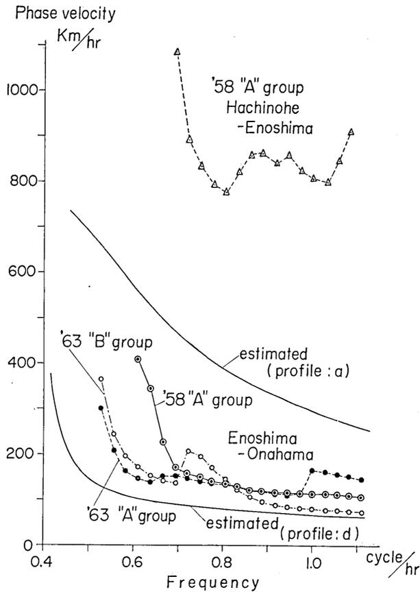
Fig. 7. Phase velocity obtained by the Fourier analysis of the dispersive wave group. The estimated dispersion curves are drawn to compare with the observation.
