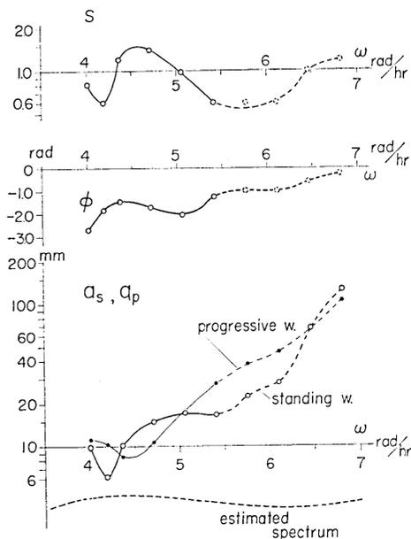
Fig. 12. Separation of the component of the oscillatory wave  $a_s$  normal to the shore and the progressive wave  $a_p$  along the shelf, with regard to Hachinohe and Enoshima in the tsunami of 1958.  $S$  shows  $|a_s|/|a_p|$  and  $\phi$  is the phase difference of two components.
