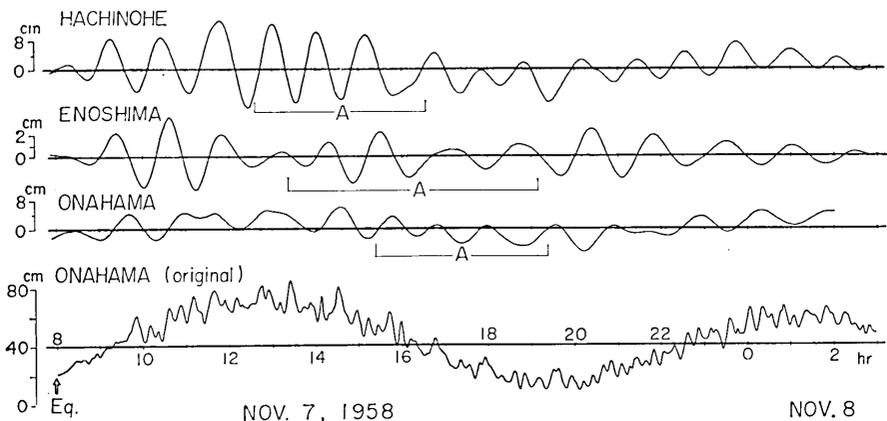
Fig. 5. Filtered and non-filtered records of the Iturup tsunami of 1958. Marks A show dispersive wave groups following the direct waves.
