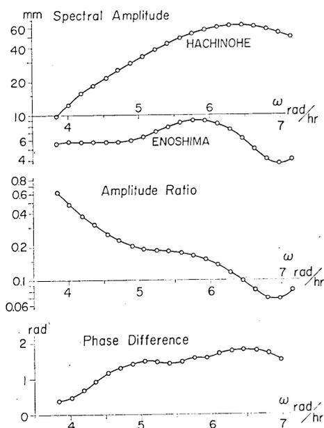
Fig. 11. Results of the Fourier analyses of the records observed at Hachinohe and Enoshima in case of the Iturup tsunami of 1958.
