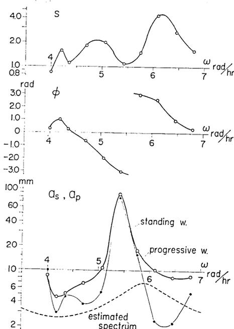
Fig. 10. Separation of the component of the oscillatory wave  $a_s$  normal to the shore and the progressive wave  $a_p$  along the shelf, with regard to Enoshima and Onahama in the tsunami of 1958.  $S$  shows  $|a_s|/|a_p|$  and  $\phi$  is the phase difference of two components.
