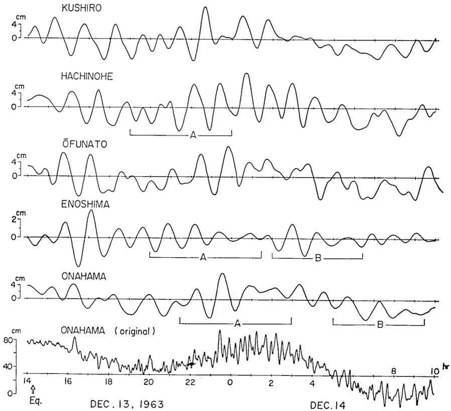
Fig. 6. Filtered and non-filtered records of the Iturup tsunami of 1963. Marks *A* and *B* show dispersive wave groups following the direct waves.
