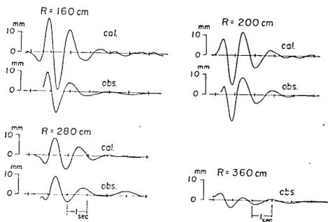
Fig. 13. Wave form at  $R=160$ , 200, 280 cm estimated from the Fourier spectrum of the wave at  $R=360$  cm in case of the experiment, being compared with the actual observed wave.  $R$  indicates the distance from the wave source to the observing point.
