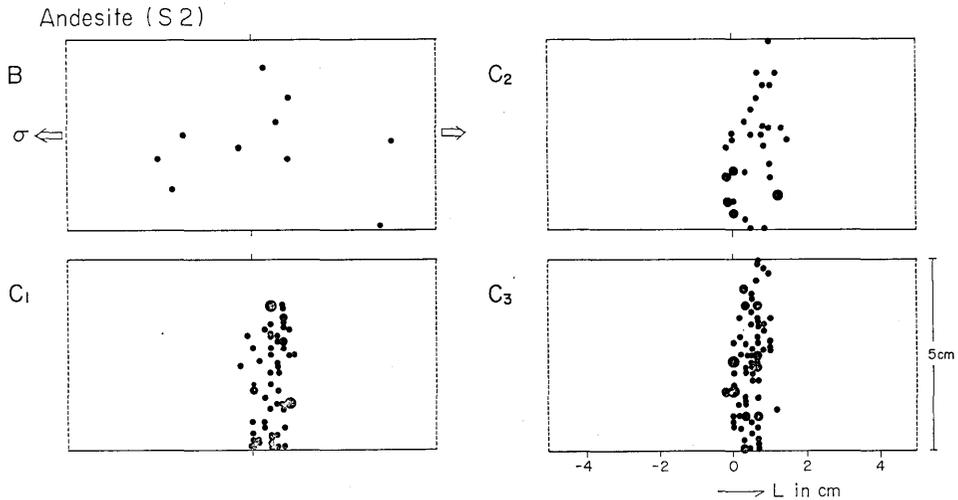
Fig. 20. Two-dimensional source locations of elastic shocks in successive stages in Shirochōba andesite (S2). Stages B, C<sub>1</sub>, C<sub>2</sub> and C<sub>3</sub> correspond to those in Fig. 19.
