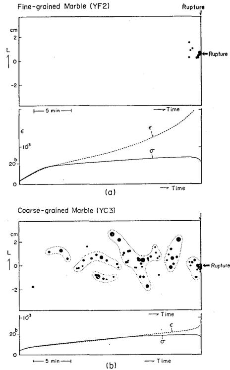
Fig. 6(a) and (b). Source locations of elastic shocks in the  $\overline{OL}$  direction as functions of time in Yamaguchi marbles. (a): fine-grained marble; (b): coarse-grained marble.  $\sigma$  and  $\epsilon$ : stress and strain at the tensile side of specimen.
