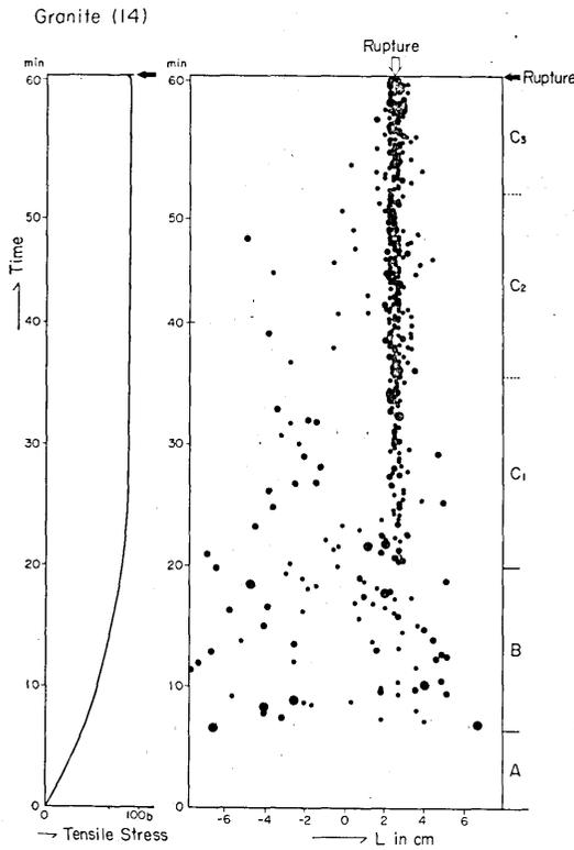
Fig. 14. Source locations of elastic shocks in the OL direction as functions of time in Inada granite (I4). Stresses at the tensile side are shown as a function of time in the left figure.
