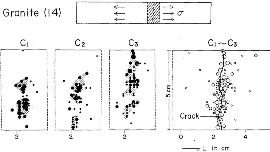
Fig. 16. Successive development of the source region of elastic shocks in the stages  $C_1 \sim C_3$  and an observed main crack pattern.
