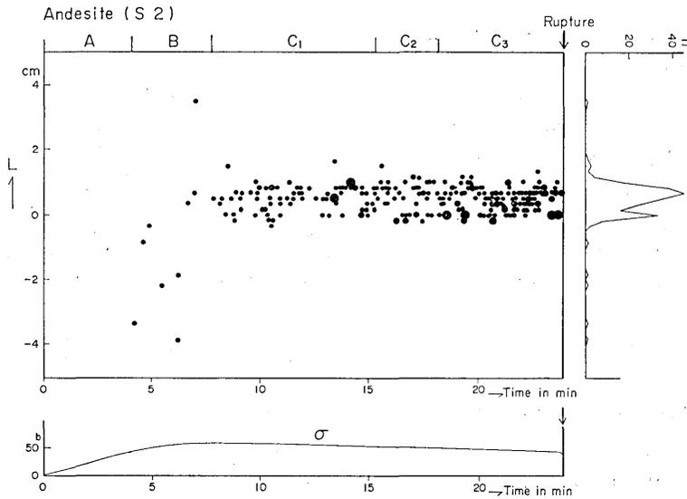
Fig. 19. Source locations of elastic shocks in the  $OL$  direction as functions of time in Shirochōba andesite (S2). A total distribution of sources is shown by a curve in the right side.  $\sigma$ : stress at the tensile side.
