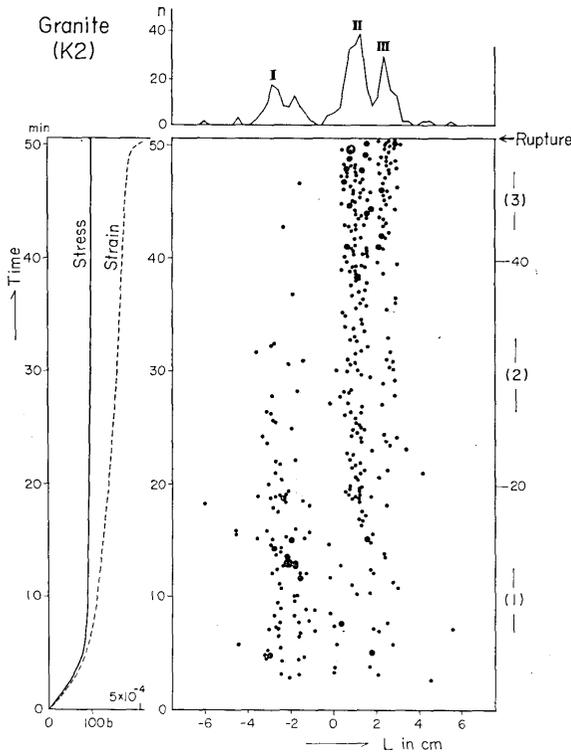
Fig. 11. Source locations of elastic shocks in the  $\overline{OL}$  direction as functions of time in Kitagi granite (K2). A total distribution of sources is shown by a curve in the upper figure. Stress and strain at the tensile side are shown as functions of time in the left figure.
