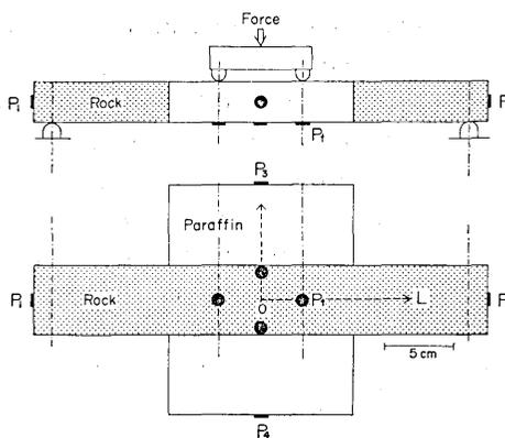
Fig. 4. The sample and transducers used in studying two-dimensional source locations of elastic shocks.  $P_1$  and  $P_2$ : transducers for shock observation;  $P_3$ : transducers for triggering synchrosopes and cameras.
