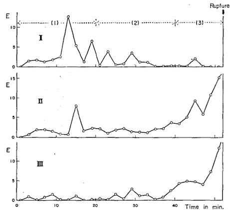
Fig. 13. Energies of elastic shocks originated from I, II and III zones as functions of time, in Kitagi granite (K2). The scale of energy is conventional.
