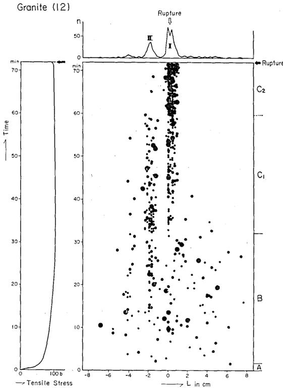
Fig. 9. Source locations of elastic shocks in the  $\overline{OL}$  direction as functions of time in Inada granite (I2). A total distribution of sources is shown by a curve in the upper figure. Stresses at the tensile side are shown as a function of time in the left figure.
