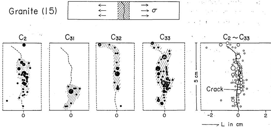
Fig. 18. Successive development of the source region of elastic shocks in the stages  $C_2$  and  $C_3$  and an observed main crack pattern.
