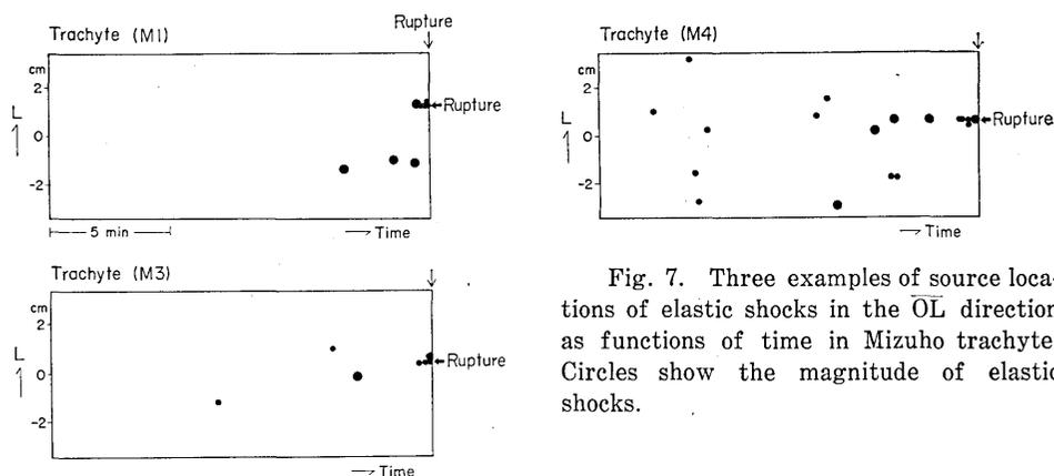
Fig. 7. Three examples of source locations of elastic shocks in the  $\bar{O}L$  direction as functions of time in Mizuho trachyte. Circles show the magnitude of elastic shocks.
