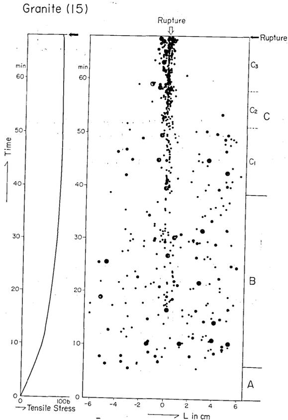
Fig. 8. Source locations of elastic shocks in the  $\overline{OL}$  direction as functions of time in Inada granite (15). A, B and C stages are indicated in the right side. Applied stresses ( $\sigma$ ) at the tensile side are also shown as a function of time in the left figure.
