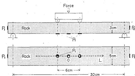
Fig. 3. The sample and transducers used in studying one-dimensional source locations of elastic shocks in rocks subjected to bending stress.  $P_1$  and  $P_2$ : transducers for shock observation;  $P_3$ : transducers for triggering synchrosopes and cameras.
