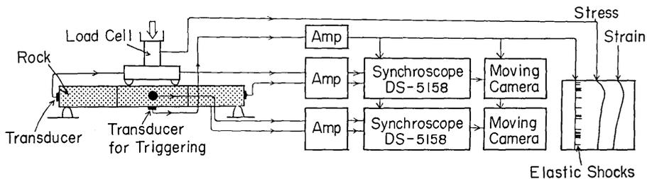
Fig. 1. Experimental system for measurement of elastic shocks caused by micro-fracturing.
