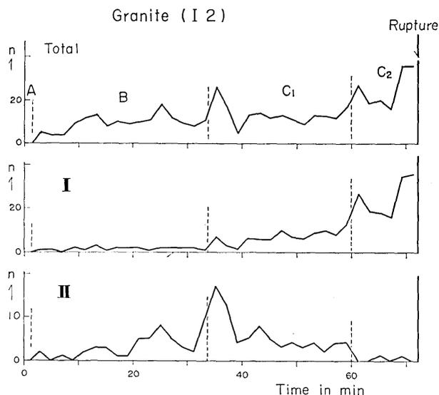
Fig. 10. Frequency curves of elastic shocks originated from the whole region (above), I zone (middle) and II zone (below). Stages A, B and C correspond to those in Fig. 9.
