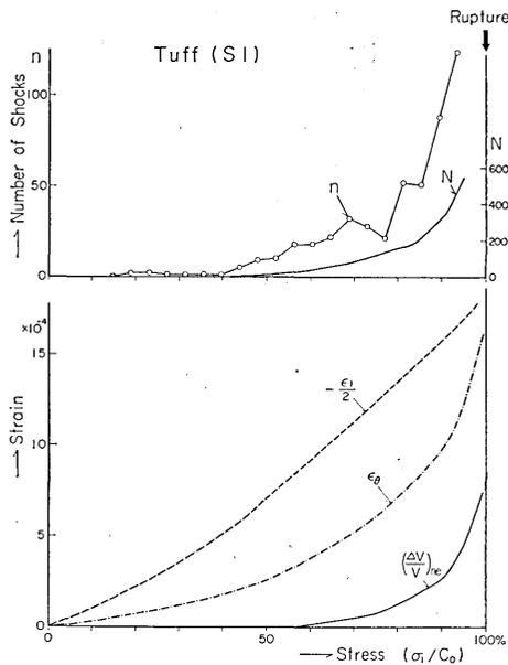
Fig. 5. Frequencies of elastic shocks (above) and strains (below) as functions of applied stress, in a uniaxial compression test of Sakuishi tuff.  $n$  and  $N$ : frequency and accumulated frequency of elastic shocks;  $\epsilon_1$  and  $\epsilon_\theta$ : axial and lateral strains;  $(\Delta V/V)_{ne}$ : non-elastic volumetric strain.
