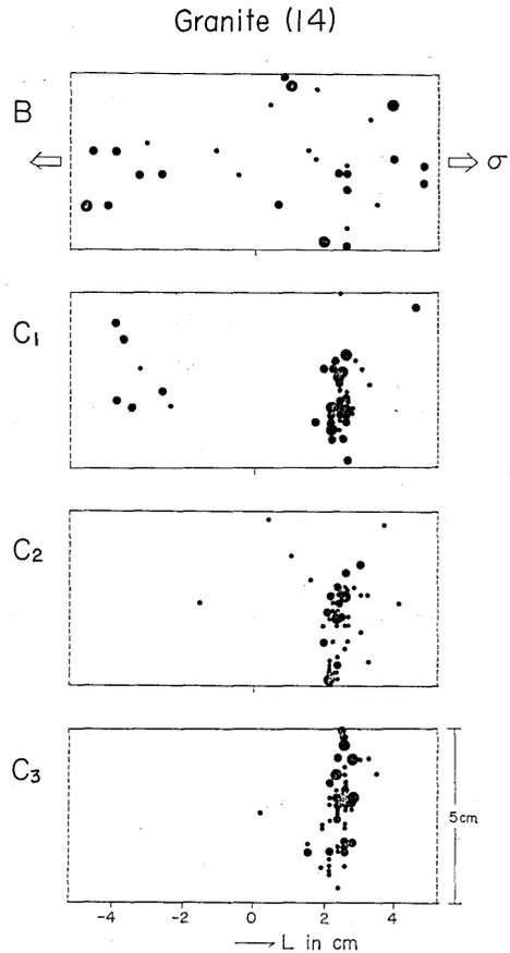
Fig. 15. Two-dimensional source locations of elastic shocks in successive stages in Inada granite (I4). Stages B, C<sub>1</sub>, C<sub>2</sub> and C<sub>3</sub> correspond to those in Fig. 14.
