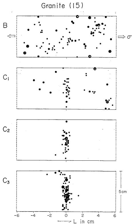
Fig. 17. Two-dimensional sources locations of elastic shocks in successive stages in Inada granite (I5). Stages B,  $C_1$ ,  $C_2$  and  $C_3$  correspond to those in Fig. 8.
