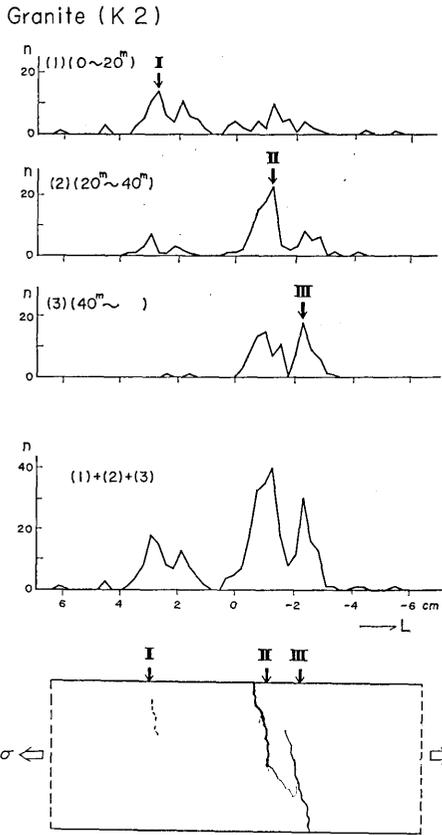
Fig. 12. Distributions of sources of elastic shocks in the  $\overline{OL}$  direction in the (1), (2) and (3) stages, and their total distribution. A lower figure shows an observed main crack pattern.
