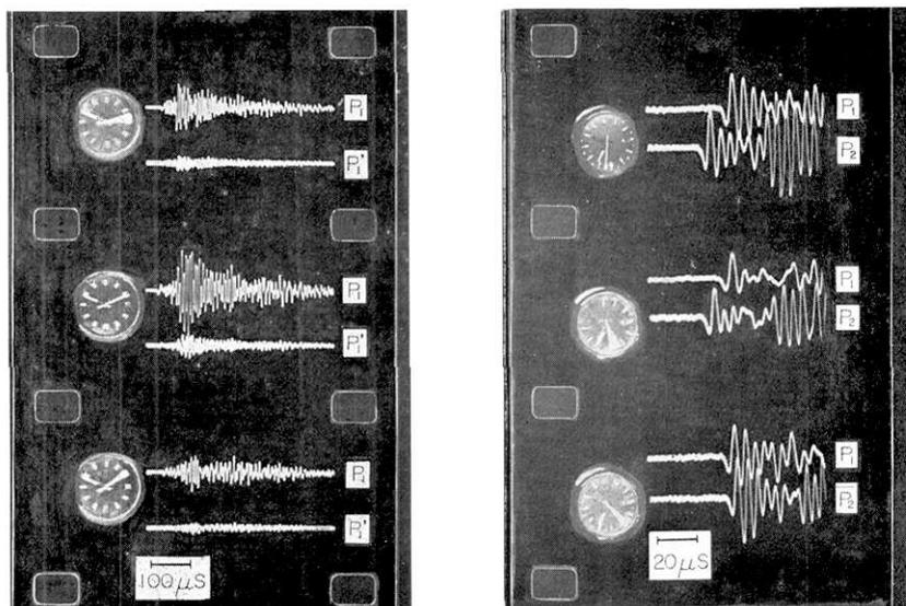
(a) Each frame shows two traces from the same transducer by different magnifications.
