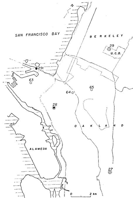
Fig. 5. Map showing locations of microtremors observation sites in the Oakland and Berkeley area.  $\odot$ ; Strong-motion seismograph site.  $\bullet$ ; Seismoscope site.
