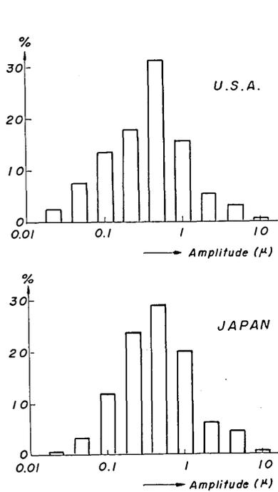
Fig. 8. Comparison of frequency distributions of amplitudes of microtremors obtained in the U. S. A. (168 sites) and Japan (800 sites).
