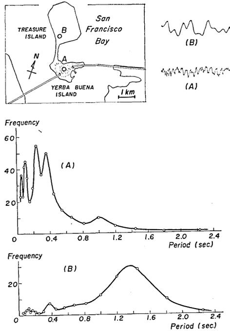
Fig. 9. Example of results of microtremors observations for different site conditions.
