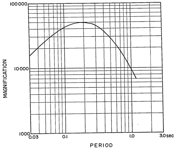
Fig. 2 Response of HES 1-0.2\* seismograph.
