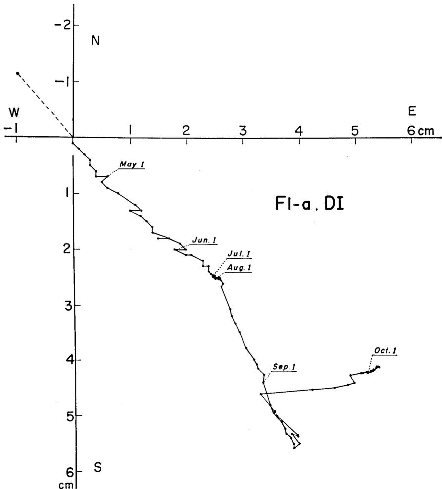
Fig. 35. Displacement path of the southwestern reference point observed at Station F<sub>1</sub>-a (D). Earlier part of this plot was given in Fig. 9(I) in the first paper.
