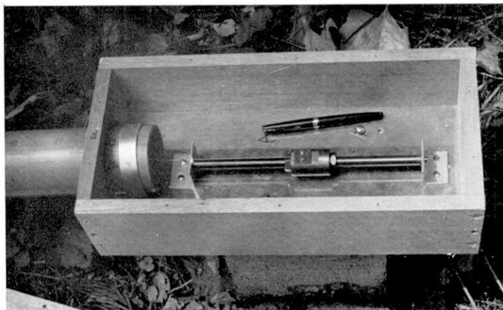
Fig. 24. Uncovered fixed end of type IV at station F<sub>4-e</sub>. An invar wire is attached to a ring whose position is adjustable along an inner rod.
