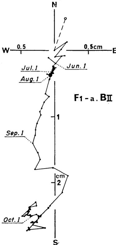
Fig. 36. Displacement path of the southeastern reference point observed at Station F<sub>1</sub>-a (B).
