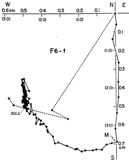
Fig. 41. Displacement path observed at Station  $F_6-f$ . Results by type III and type V are represented by solid circles connected by solid and dotted lines, respectively. Scale for the latter is parenthesized.
