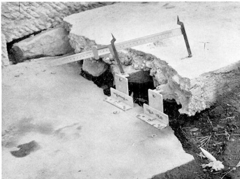
Fig. 27. Raised reference points of type Ic-w at Station F<sub>1-a</sub> (A). Vertical displacement along crack A made the former measurement impossible. Photograph taken March 9. Vertical view is given in Fig. 13.
