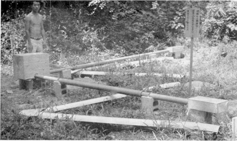
Fig. 22. Complete view of station F<sub>4-e</sub> as seen from the east. Three sets of measuring instruments are installed, of which the smaller two are type III-v and the overlapping long one type IV. Relation to ground cracks is shown in Fig. 29.
