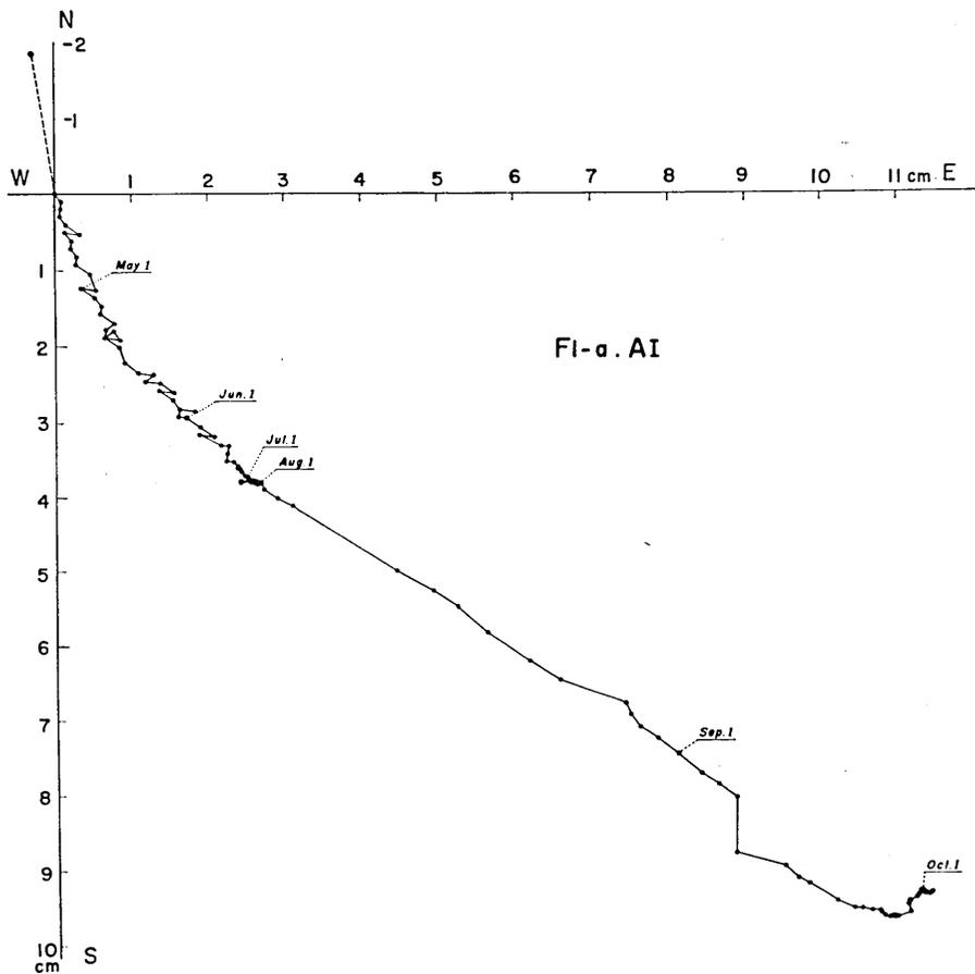
Fig. 33. Displacement path of the southwestern reference point observed at Station F1-a (A). Earlier part of this plot was given in Fig. 8(I) in the first paper.
