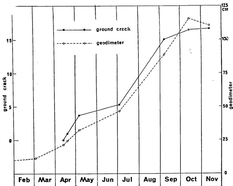
Fig. 49. Comparison of the time rate of displacement. Solid circle: measurement across a ground crack, at F<sub>1</sub>-a (Fig. 12), simplified from F<sub>1</sub>-a-AI in Fig. 42. Open circle: electro-optical measurement along a base line about 3 km long, between Mt. Minakami and Sorobeku (Fig. 12).
