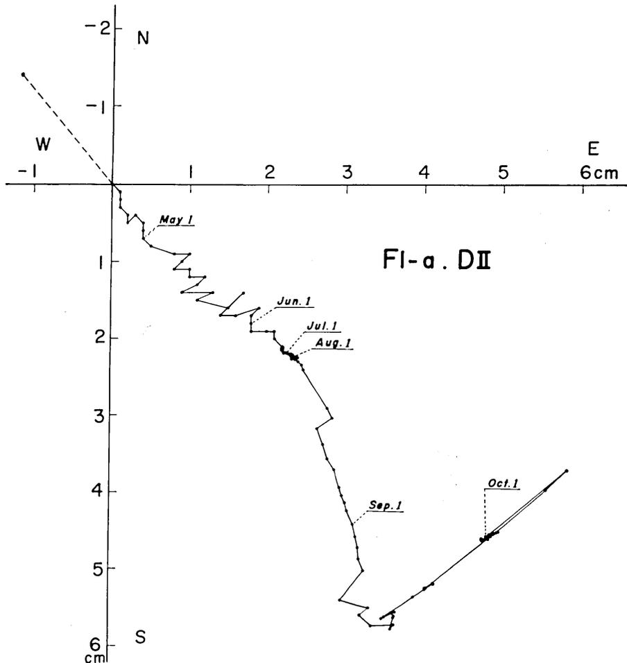
Fig. 34. Displacement path of the southeastern reference point observed at Station F1-a (D). Earlier part of this plot was given in Fig. 9(II) in the first paper.
