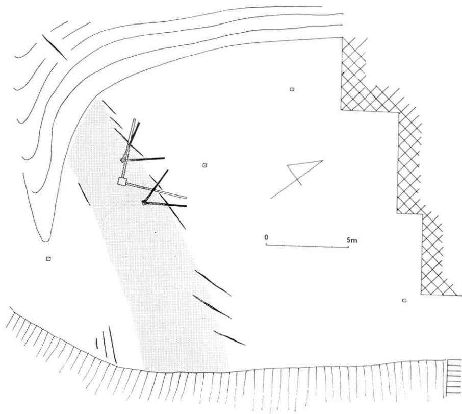
Fig. 29. Sketch map of Station F<sub>4</sub>-e in the yard of a shrine. Three sets of measuring instruments are shown. Larger one is of type IV-v and the smaller ones are of type III-v. Stippled area is a graben-like depression of about 15 cm in depth developed in August and September, 1966.
