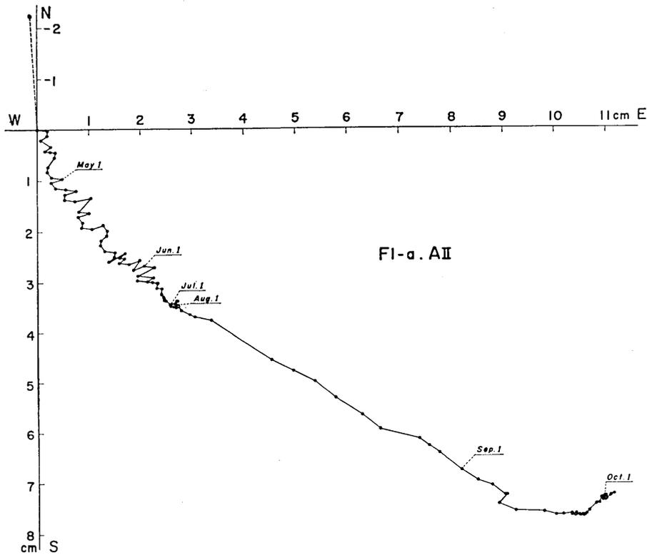
Fig. 32. Displacement path of the southeastern reference point observed at Station F<sub>1-a</sub> (A). Earlier part of this plot was given in Fig. 8(II) in the first paper.
