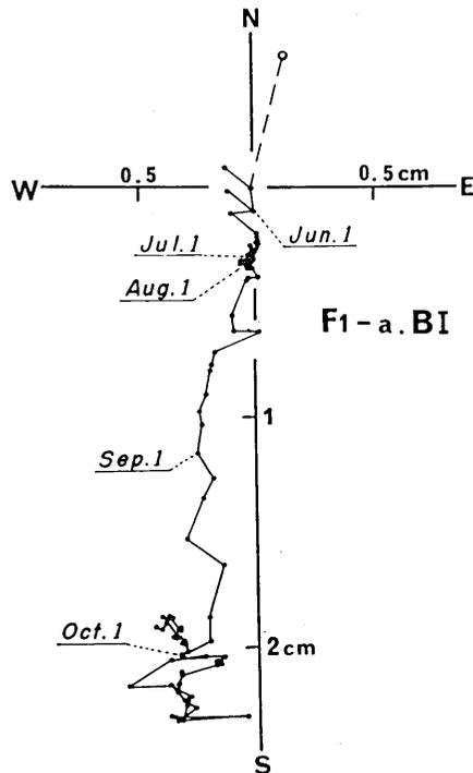
Fig. 37. Displacement path of the southwestern reference point observed at Station F<sub>1</sub>-a (B).
