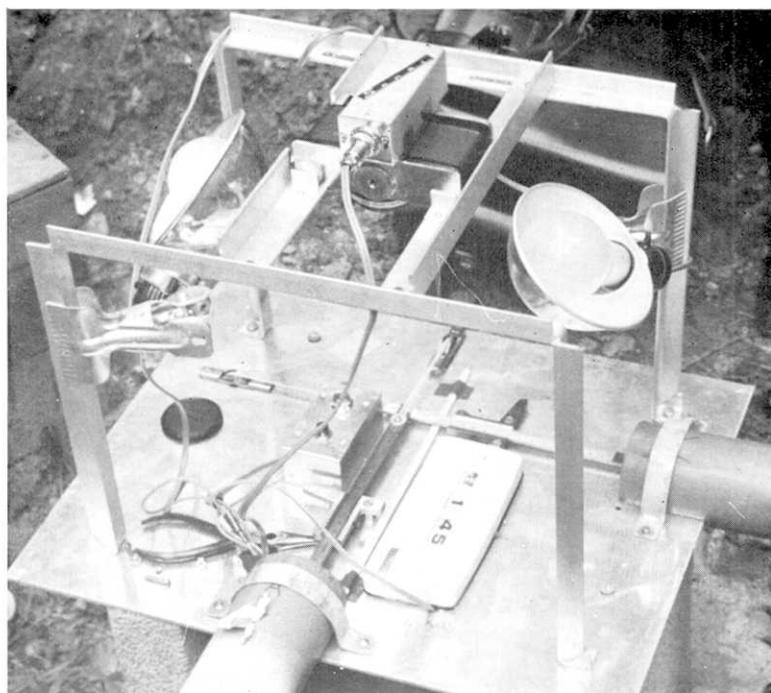
Fig. 25. Uncovered recorder of type IV. An automatic camera is positioned on the top.
