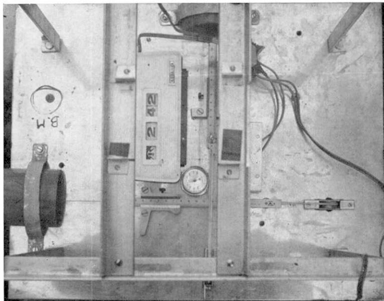
Fig. 26. Vertical view of instrument board of the recorder of type IV. Two vernier callipers, a clock and a thermometer are arranged. Automatic camera is removed.
