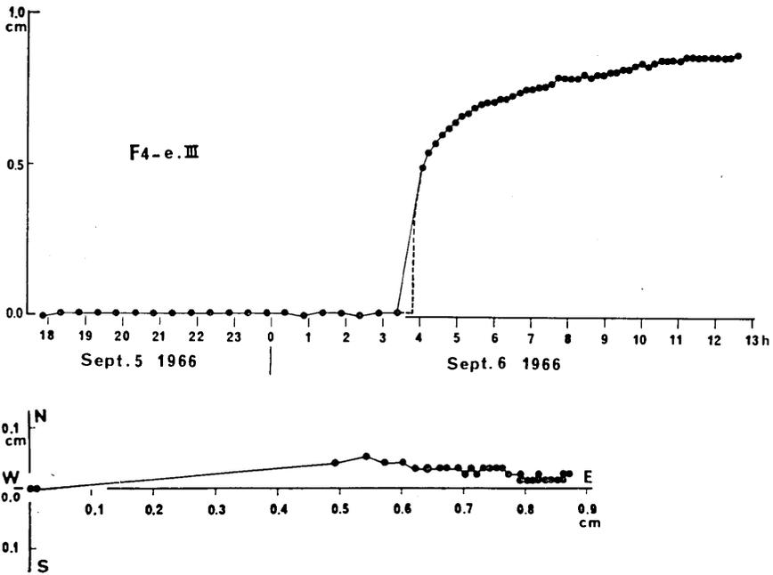
Fig. 40. Displacement path (below) and amount of displacement (above) before and after a large shock ( $M=5.0$ ) observed by type IV at Station  $F_4-e$ .
