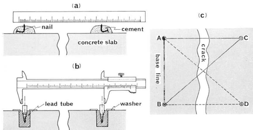
Fig. 17. Structure of reference points used in type Ib (a) and type Ic (b) and their arrangement (c).
