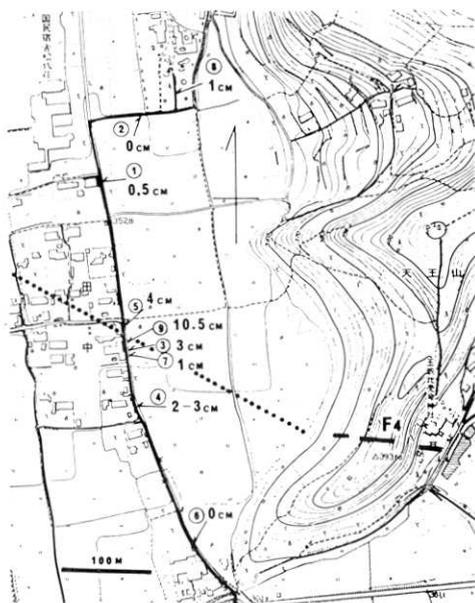
Fig. 47. Location of damaged water pipe to Ichiyōkan Hotel. Thick line shows the water line. Arrows indicate positions of damage, and distances pulled apart by the damage. Numbers in circle are common to those in Table 5.
