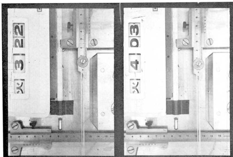
Fig. 30. Photograph taken by type IV just before (3 h 22 m) and after (4 h 03 m) a large shock ( $M=5.0$ , 3 h 37 m, September 6, 1966) recording an acute displacement. Lower callipers (NW-SE) show extension of 3.1 mm, upper ones (NE-SW) contraction of 3.7 mm, indicating lateral displacement during the 41-minutes interval between photographs. Analysed data are given in Fig. 40. The displacement may have taken place in far less than 41 minutes.
