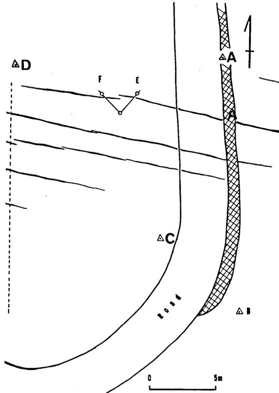
Fig. 31. Sketch map of Station F<sub>c</sub>-f. A, C and D are reference points used by a method of type V. E and F are free ends of type III-v.
