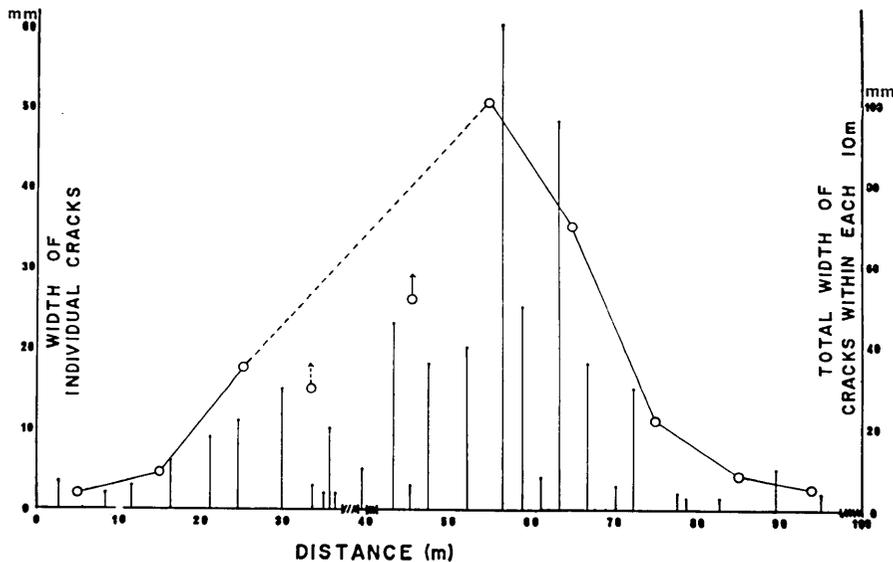
Fig. 46. Distribution of open cracks along a roadside ditch. Vertical lines indicate the location and separation of individual open cracks. Open circles represent accumulated sum of separation for each 10 metres. Hatched parts of the horizontal line show the places where the concrete ditch is either discontinuous or incapable of being observed due to obstacles.
