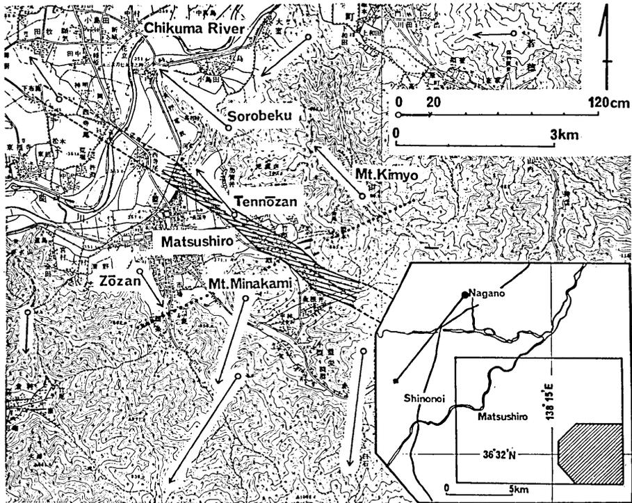
Fig. 50. Vectors representing horizontal displacement, 1904-1966, in the Matsushiro area.<sup>11)</sup> A circle and an arrow in the smaller map indicate fixed triangulation point and direction. Hatched zone in the larger map shows location of the assumed buried fault according to surface evidence (cf. Fig. 12).
