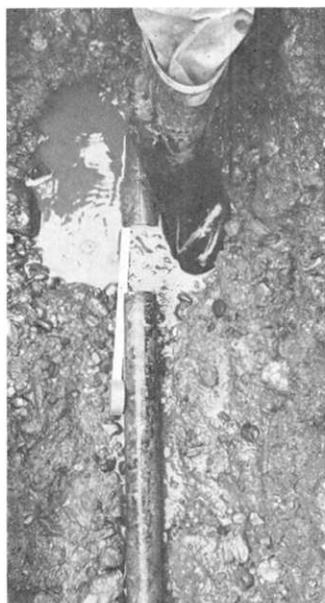
Fig. 48. Photograph showing the pull apart damage of a water pipe in shallow underground. Number 9 in Fig. 47 and Table 5. The distance is 10.5 cm. Photograph taken by Mr. Isao Kasuga, on September 9, 1966.
