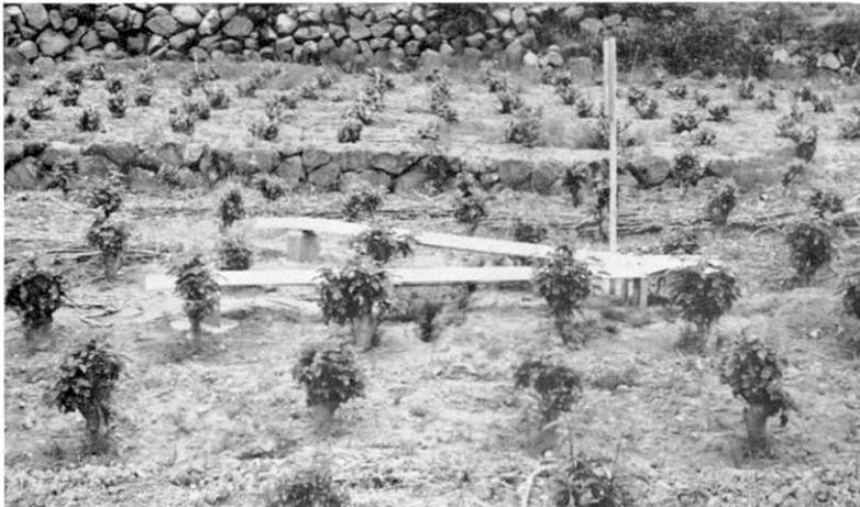
Fig. 21. Displacementmeter of type IIb-v installed in a mulberry field at Station F<sub>3</sub>-d. Relation to ground cracks is shown in Fig. 28.
