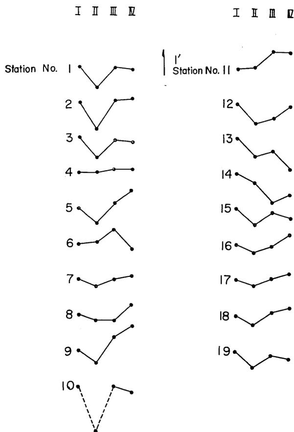
Fig. 7. Changes in the geomagnetic dip at each station over the Matsushiro area as observed by repeating magnetic dip surveys.
