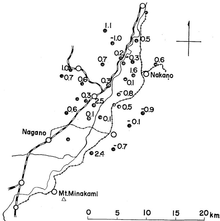
Fig. 9. Changes in the geomagnetic dip over the Nakano-Susaka area during the period from Survey II and Survey III.
