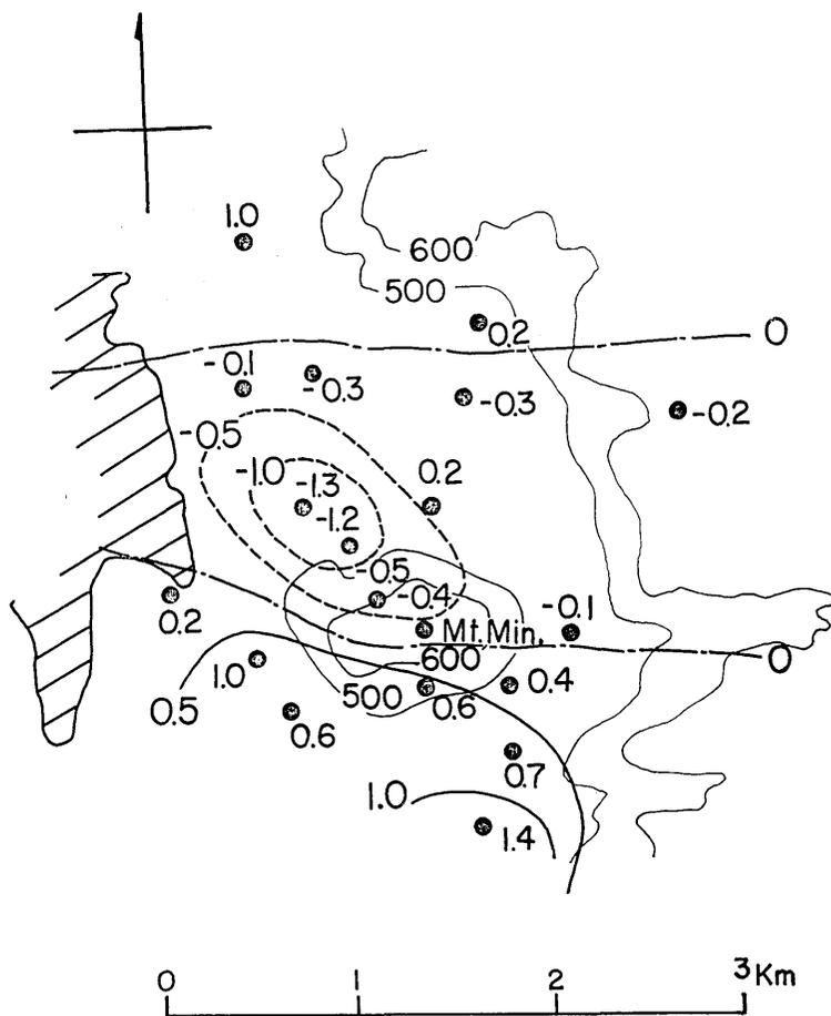
Fig. 8. Changes in the geomagnetic dip over the Matsushiro area during the period from Survey I to Survey IV.
