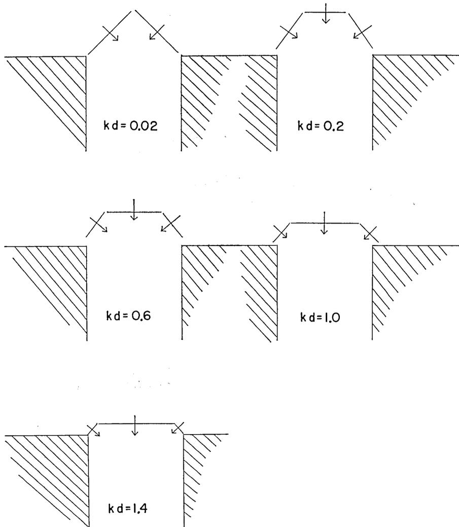
Fig. 9. A variation of forms of crest lines versus  $kd$  (arrows stand for the direction of propagation of waves).
