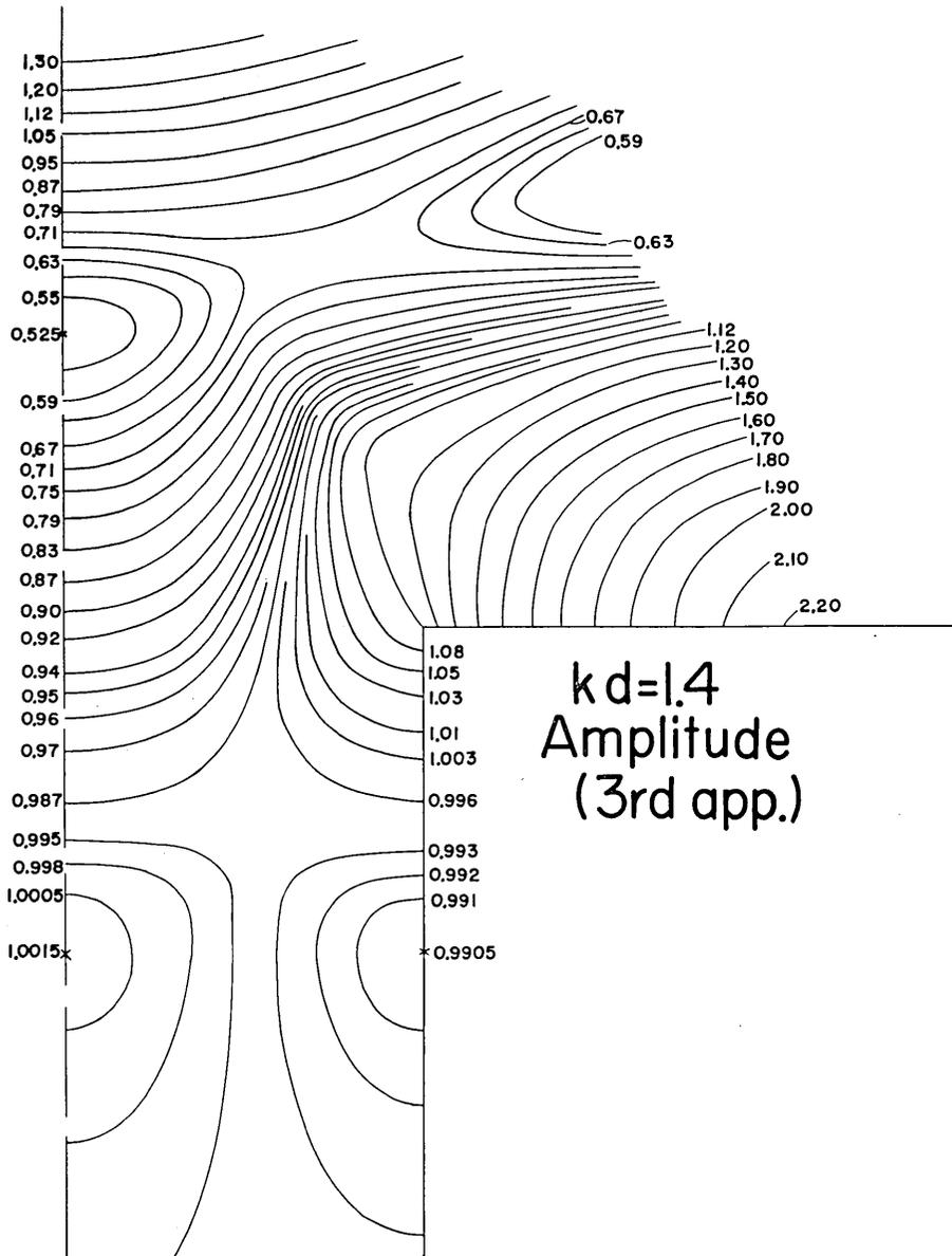
Fig. 16. A variation of amplitude around an estuary for  $kd=1.4$  (the stated values stand for  $|\zeta|$ , which are computed by the theory of the third approximation).
