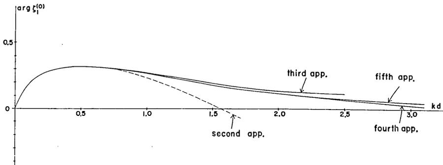
Fig. 3. A variation of the phase of the advancing mode in the canal versus  $kd$ .
