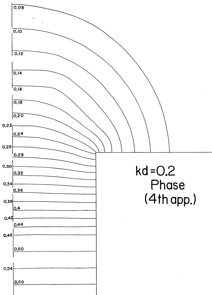
Fig. 5. Isolines of phase around an estuary for  $kd=0.2$  (the stated values stand for  $\arg \zeta$ ).
