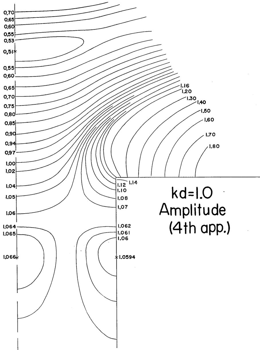
Fig. 12. A variation of amplitude of waves around an estuary for  $kd=1.0$  (the stated values stand for  $|\zeta|$ ).
