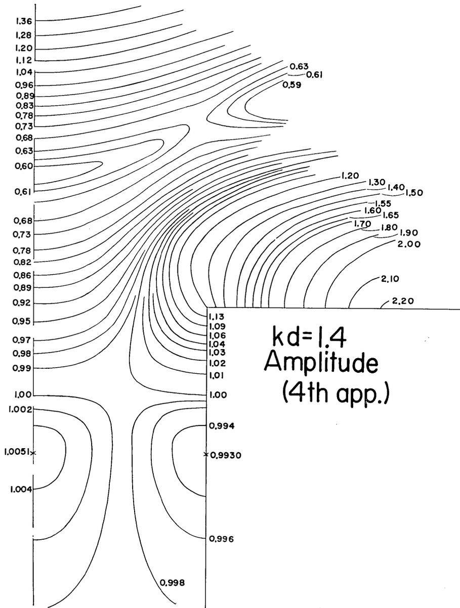
Fig. 13. A variation of amplitude of waves around an estuary for  $kd=1.4$  (the stated values stand for  $|\zeta|$ ).
