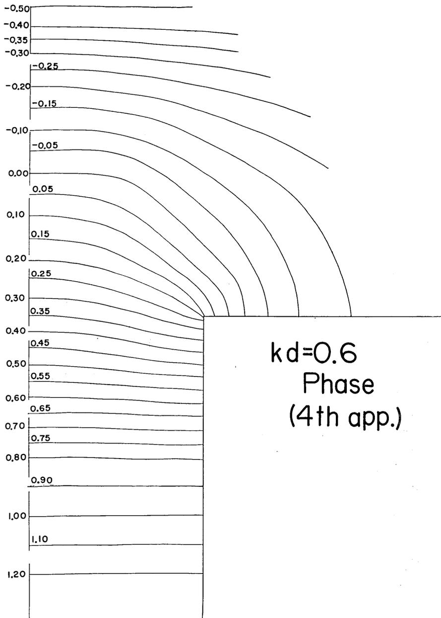
Fig. 6. Isolines of phase around an estuary for  $kd=0.6$  (the stated values stand for  $\arg \zeta$ ).
