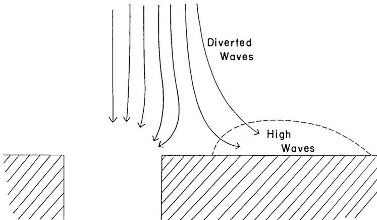
Fig. 20. A figurative explanation of high waves along the straight coast.
