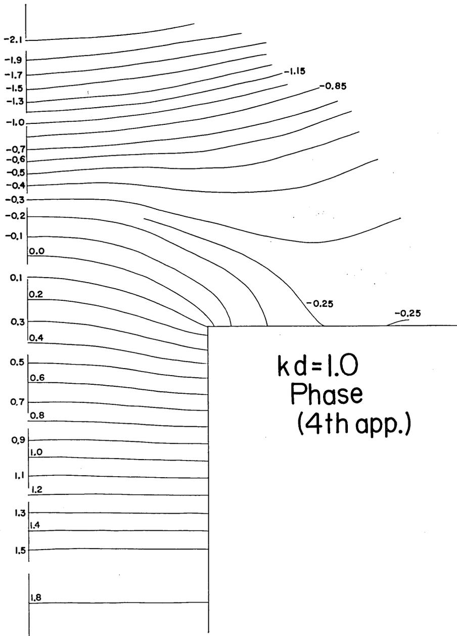
Fig. 7. Isolines of phase around an estuary for  $kd=1.0$  (the stated values stand for  $\arg \zeta$ ).
