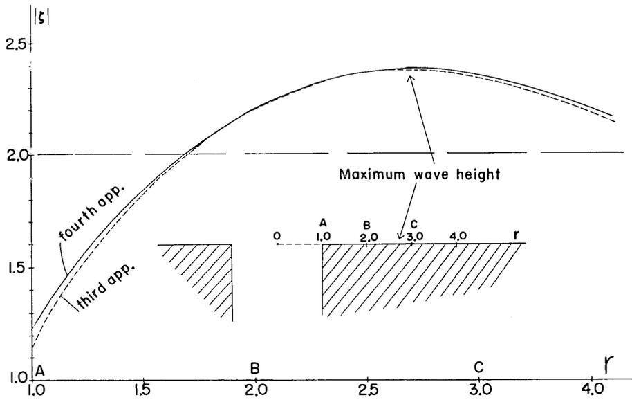
Fig. 19. A variation of the amplitude of waves for  $kd=1.4$  along the straight coast.
