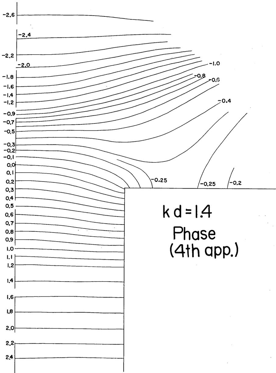
Fig. 8. Isolines of phase around an estuary for  $kd=1.4$  (the stated values stand for  $\arg \zeta$ ).
