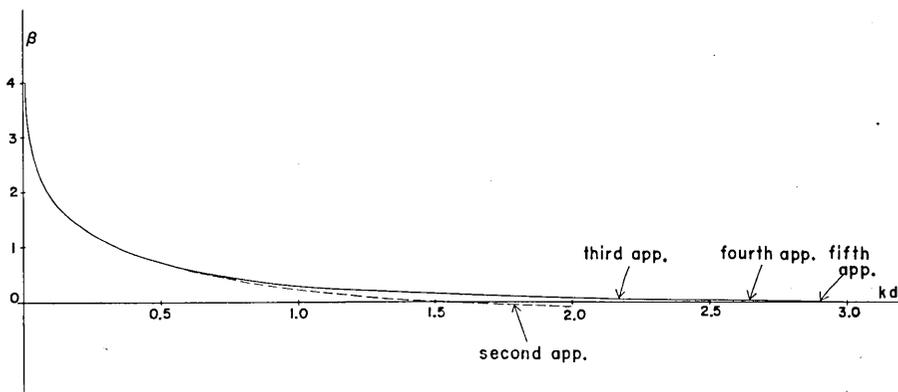
Fig. 4. A variation of a supposed origin of the  $\cos(\omega t + ky)$ -type wave in the canal versus  $kd$ .
