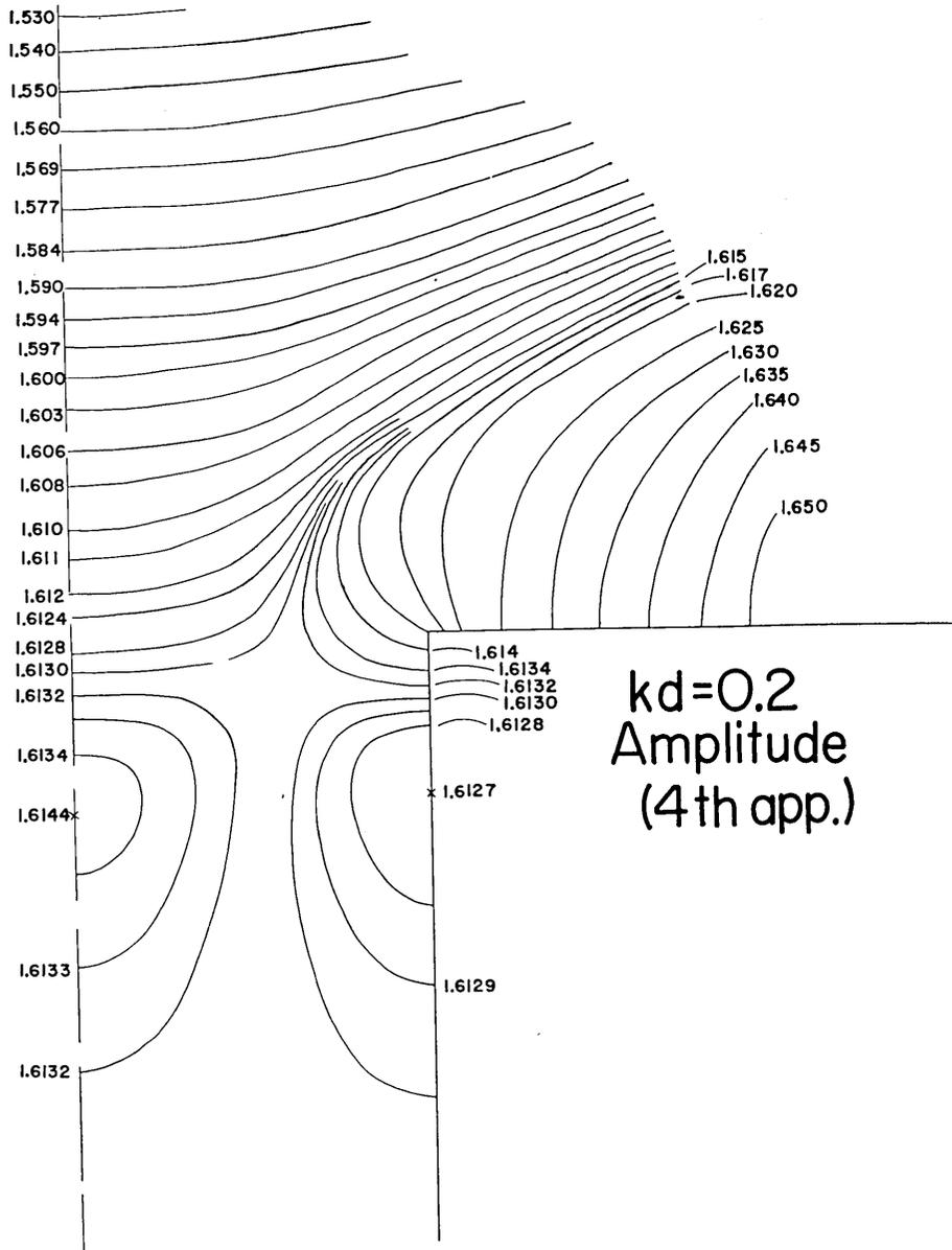
Fig. 10. A variation of amplitude of waves around an estuary for  $kd=0.2$  (the stated values stand for  $|\zeta|$ ).
