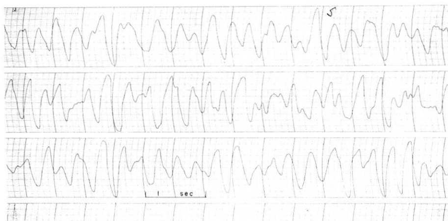
Fig. 54. Volcanic tremor recorded by the tripartite network during the October eruption by means of a 3-channel magnetic tape recorder.
