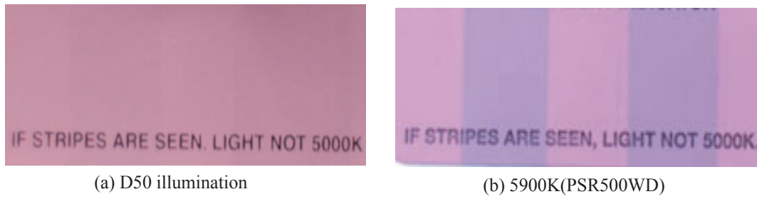
Figure 2.5: Light indicator strips under D50 (left) and 5900K (right). Viewed under 5000K or D50 standardized lighting conditions, light indicator strips will appear to be a solid color.
