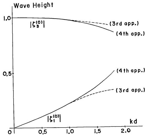
Fig. 2. Variations of amplitudes of reflected and advancing waves.
