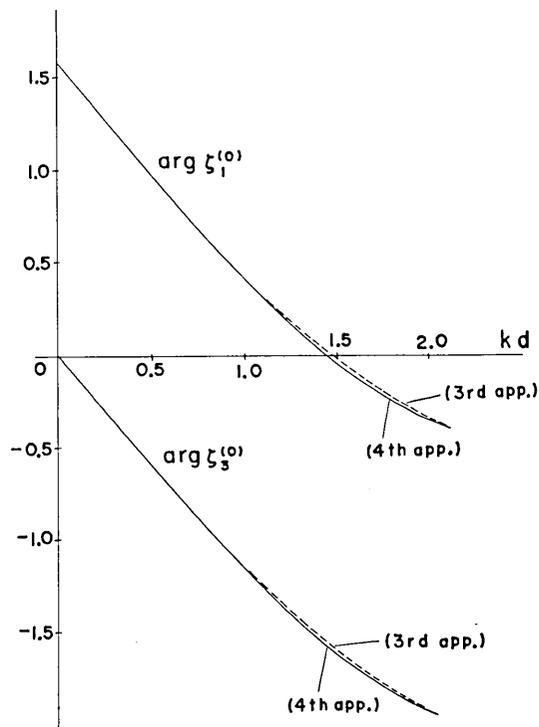
Fig. 3. Variations of phases of reflected and advancing waves.
